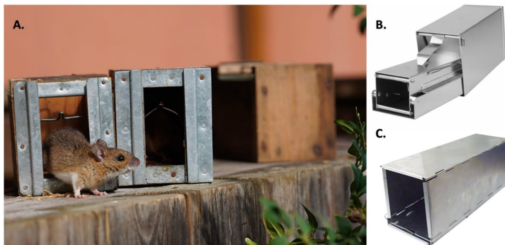
Fig. 4 A Housemade wooden trap contains a small metal platform internally, which, when triggered, causes a metal door to close (image shows a wood mouse— Apodemus sylvaticus ). B Longworth trap; C Sherman trap
