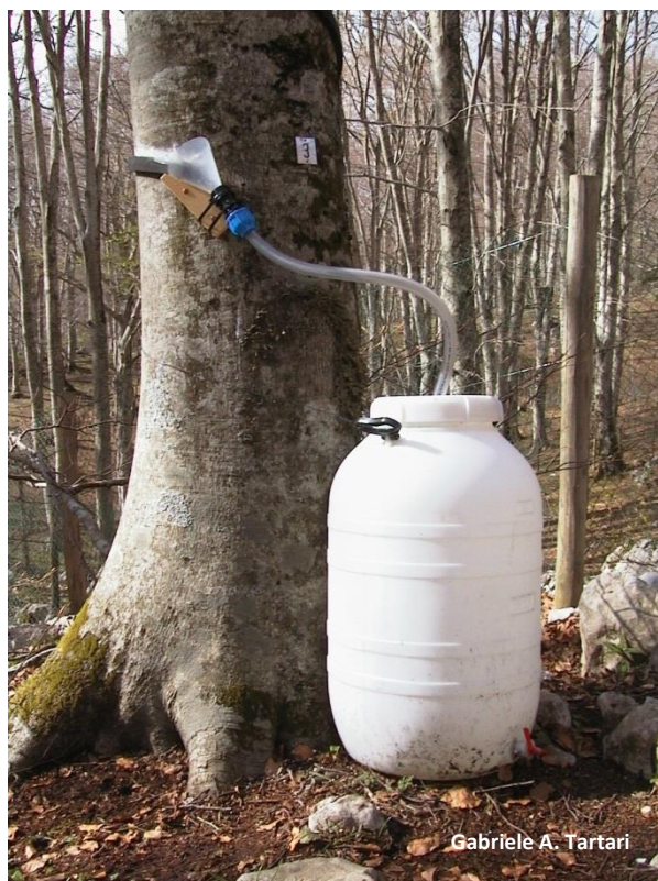
Figure 4-2. Stemflow sampler on a beech stem in Italy.
