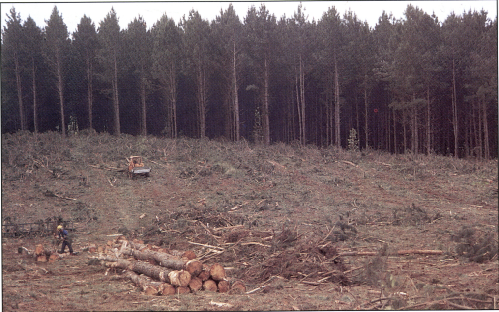
Figure 12. A grapple skidder, equipped with a safety frame, delimiting whole pine trees by backing its load through a delimiting gate at a landing site in the state of Santa Catarina. Bucking to assortments is made manual by chainsaw. (Photo: Jari Parviainen)
