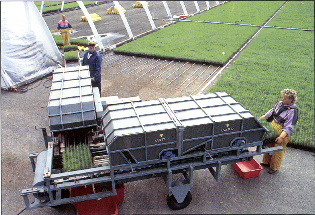
Figure 14. Production of VAPO-pine seedlings in the plastic greenhouse in Finland. The roots and the peat sheet are pruned vertically on four sides using circular sawblades. (Photo: Leo Tervo)
