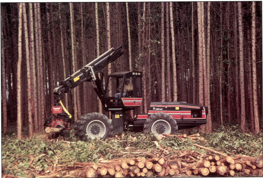
Figure 13. A typical Finnish one grip harvester operating by clear cutting in a mature eucalyptus stand in Brazil. (Photo: Olli Eeronheimo)
