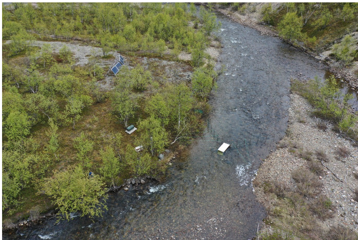
Figure 7. Simsonar FC stereo camera system installed to the River Gálddašjohka/Kalddasjoki. The white box in the middle of the river is the camera tunnel unit. Guiding fences goes from the tunnel unit downstream to both shores. Data recording and solar power systems are situated on the shore (left hand side). Photo: Mikko Kytökorpi.
