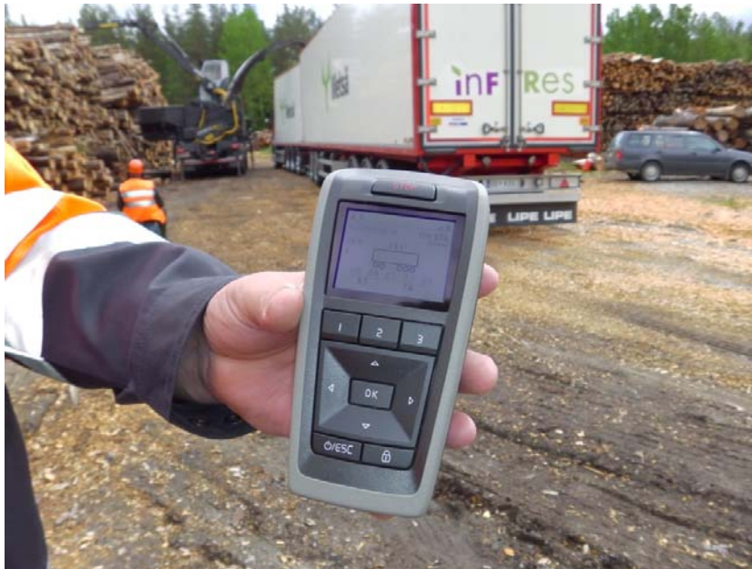
Figure 6 – The axle mass monitoring device (Photo: Antti Asikainen/Luke).
