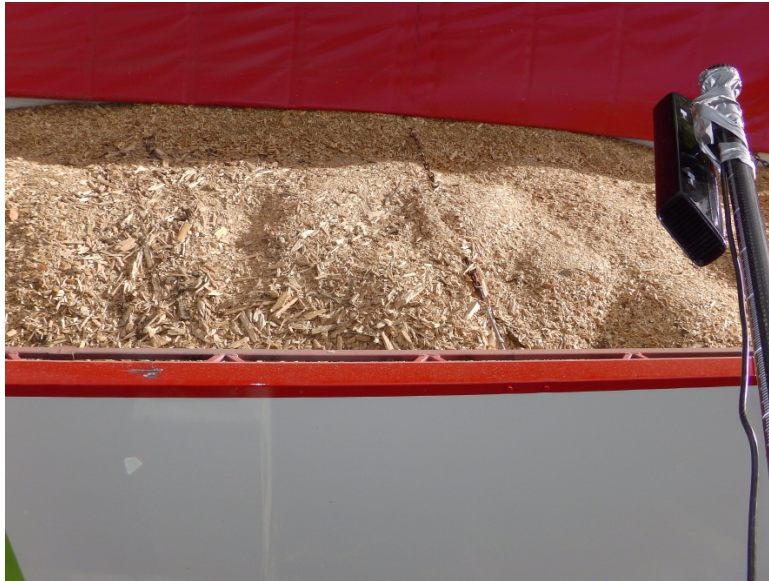
Figure 10 – The Microsoft Kinect sensor was installed at the end of the rod and it was moved manually over the container (Photo: Antti Asikainen/Luke).
