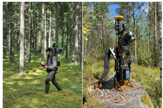
Figure 3 Illustration of the mobile laser scanning setup including a Faro Orbis scanner paired with a Trimble DA2 GNSS receiver.
