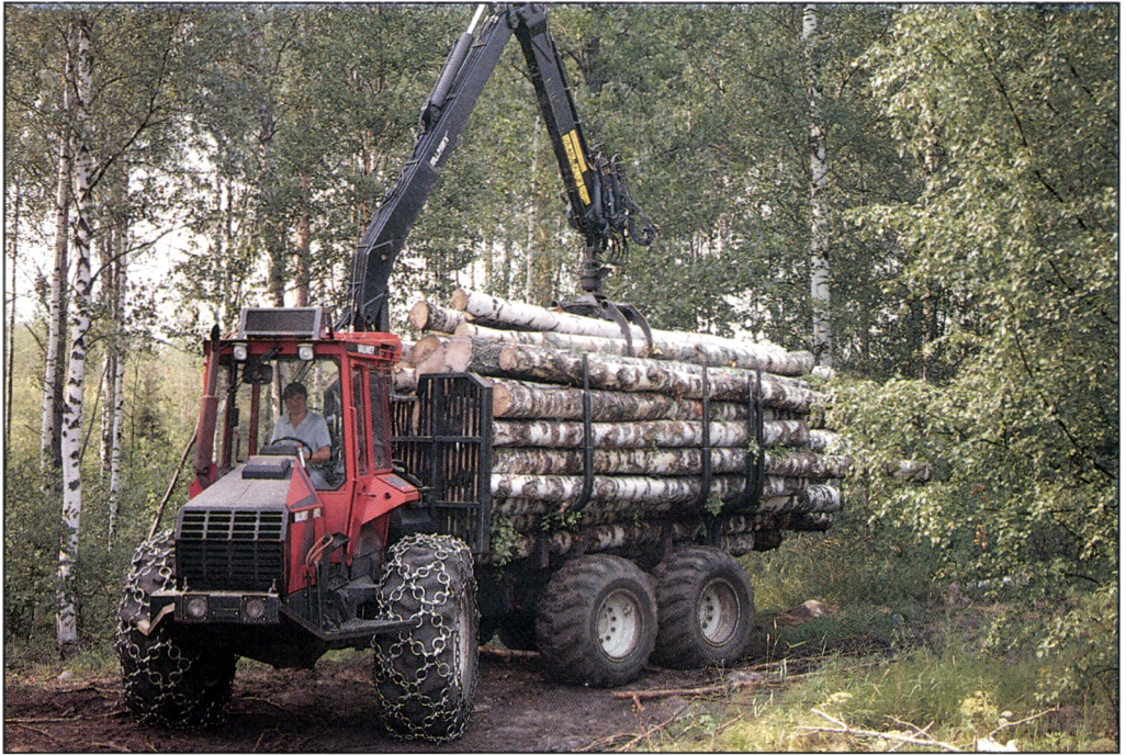
Figure 17. In Finland the log-length system is characterized by the use of load-carrying, self-loading special forwarders for off-road transport. A Valmet 862 forwarder hauling birch veneer logs (Photo Erkki Oksanen).
