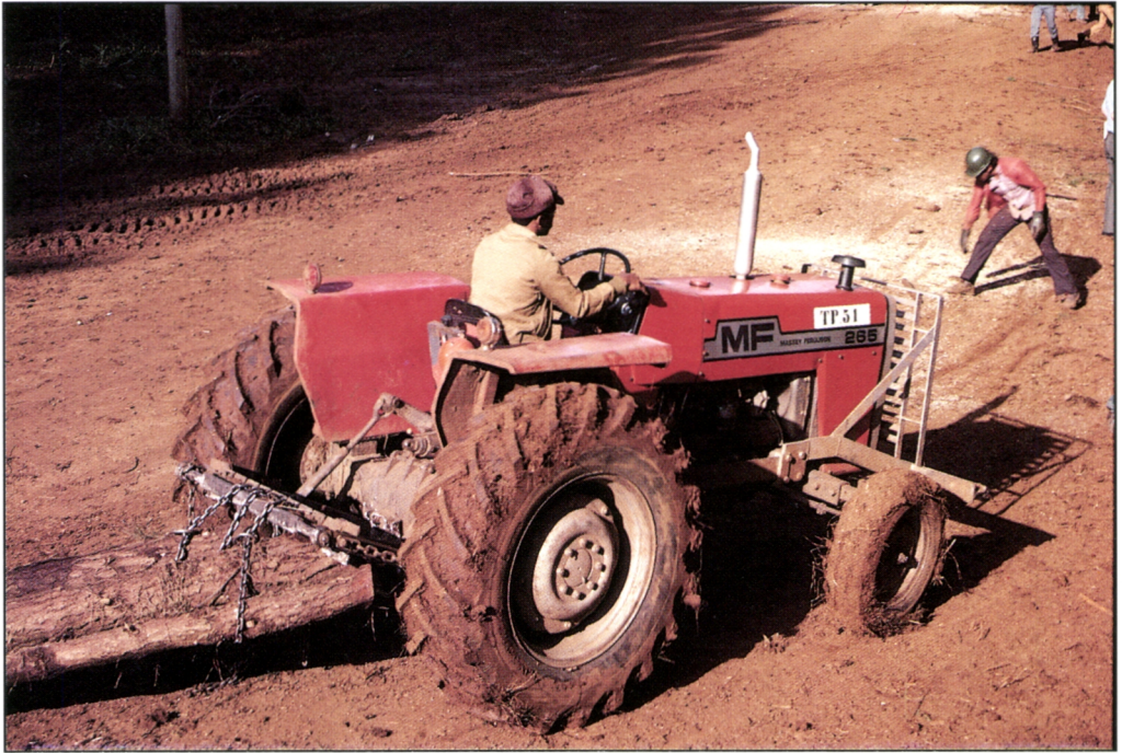
Figure 8. Simple Brazilian equipment for ground skidding. A steel bar with a set of chains attached to the three-point linkage of a Massey Ferguson farm tractor. The driver is not protected with a safety frame (Photo Pentti Hakkila).
