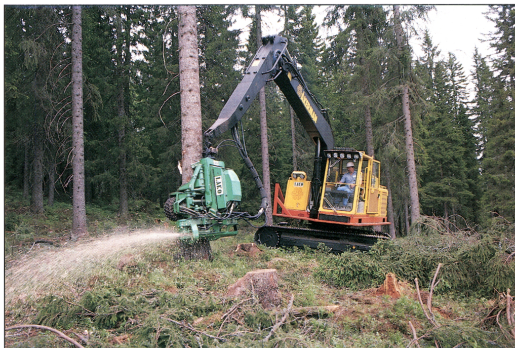
Figure 21. A Lako one-grip harvester head mounted on an Åkerman excavator. Clear-cutting a mature spruce stand in Finland (Photo Arctic Forest Machines).
