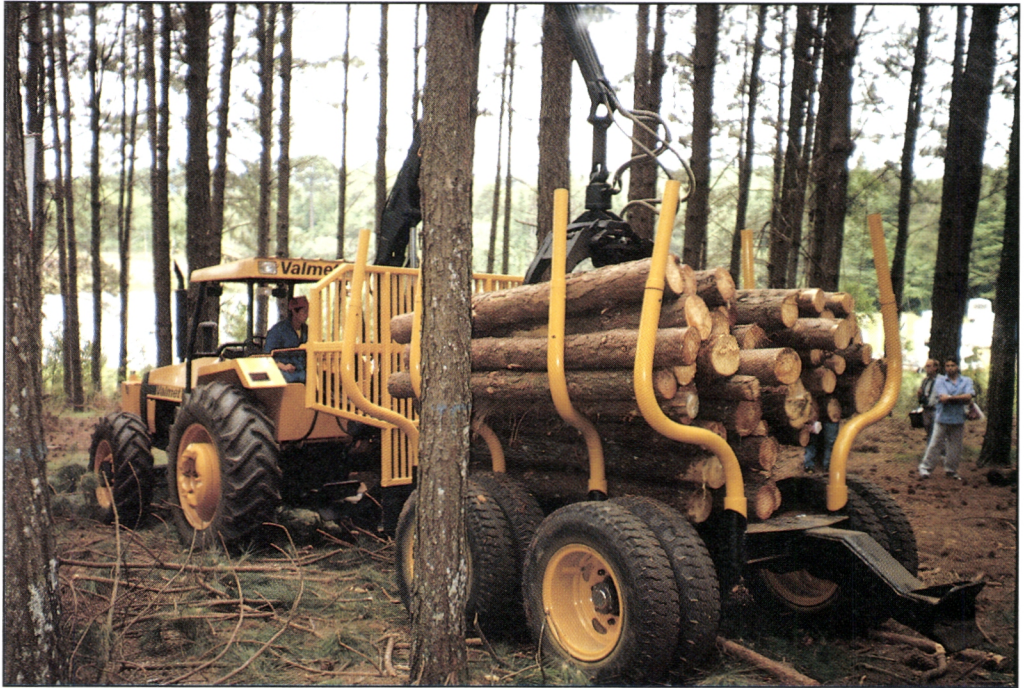
Figure 11. A Valmet farm tractor equipped with a safety frame, trailer and crane for off-road transport in Brazil. (Photo Jorge Malinovski).
