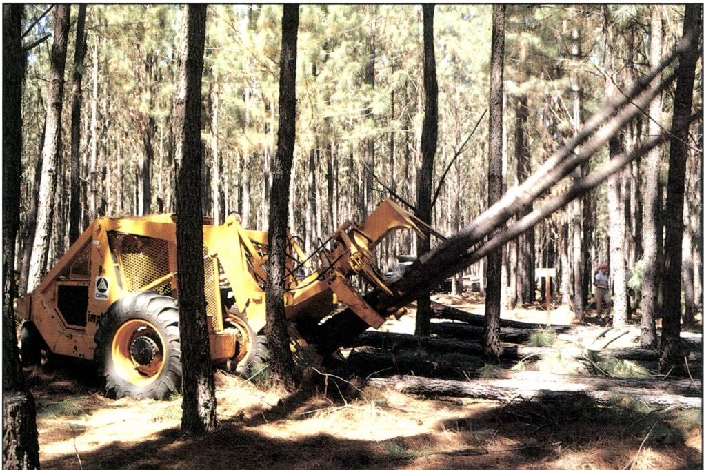
Figure 5. Implenor Bell feller-buncher in a late thinning operation in Brazil (Photo Jorge Malinovski).
