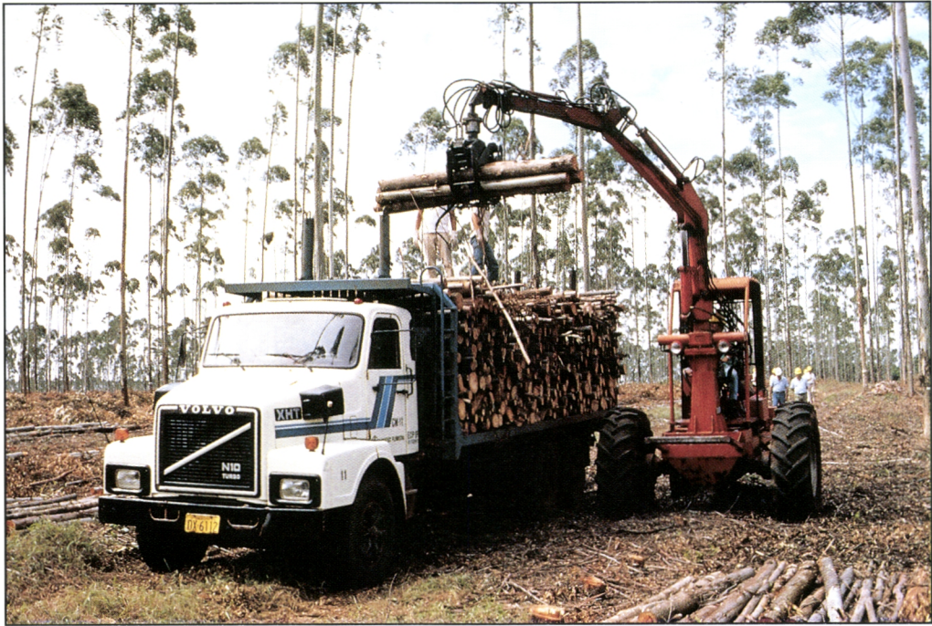
Figure 13. Loading a Volvo timber truck with a separate tractor at the logging site in Brazil (Photo Jorge Malinovski).
