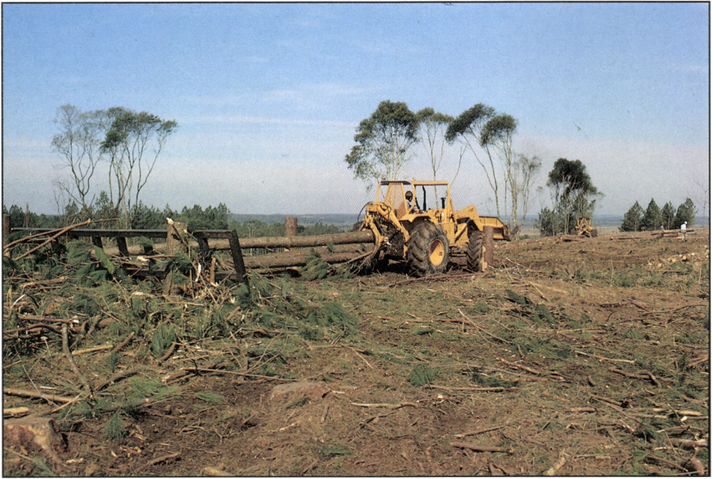
Figure 9. A grapple skidder, equipped with a safety frame, delimiting whole pine trees by backing its load through a delimiting gate at a landing site in Brazil (Photo Jorge Malinovski).
