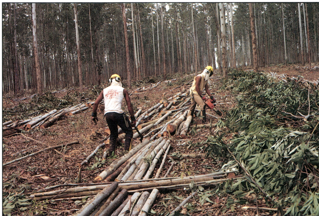
Figure 6. The log-length system in a clear-cutting operation of a eucalyptus stand in Brazil. A team of two cutters, one using a chainsaw and the another using an ax (Photo Jorge Malinovski).
