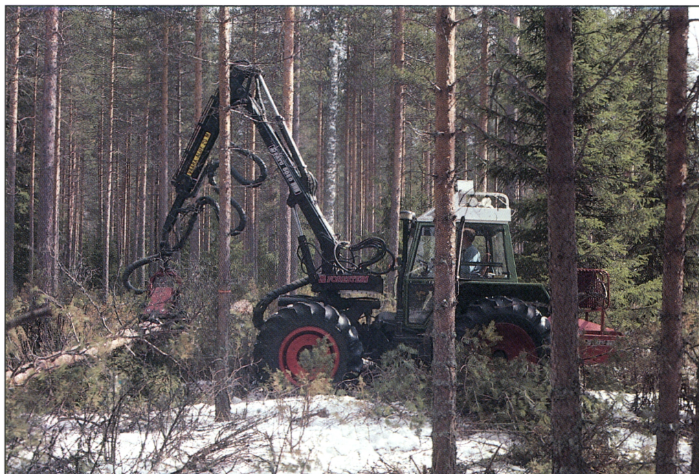
Figure 20. A Patu one-grip harvester head mounted on a Fendt farm tractor. Early thinning of a pine stand in Finland (Photo Seppo Rynänen).
