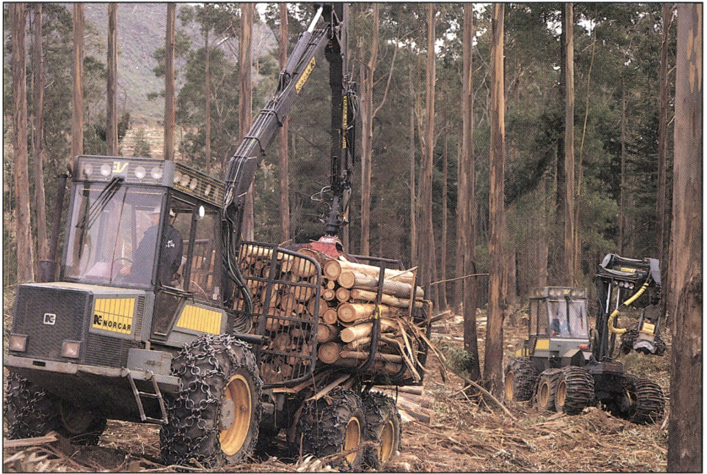
Figure 23. A fully mechanized logging system in clear-cutting of a eucalyptus stand in Chile. Norcar HS 15 harvester and Norcar S 15 forwarder (Photo Kristian Stén).
