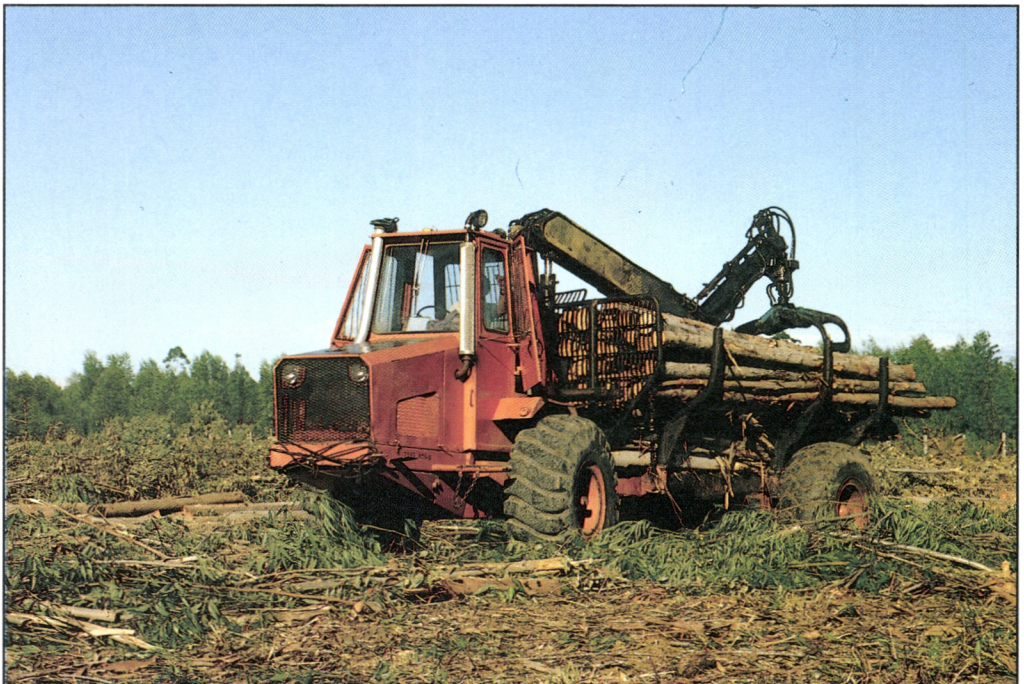
Figure 12. A four-wheel Engesa forest tractor forwarding long pulpwood logs of eucalyptus in Brazil (Photo Jorge Malinovski).
