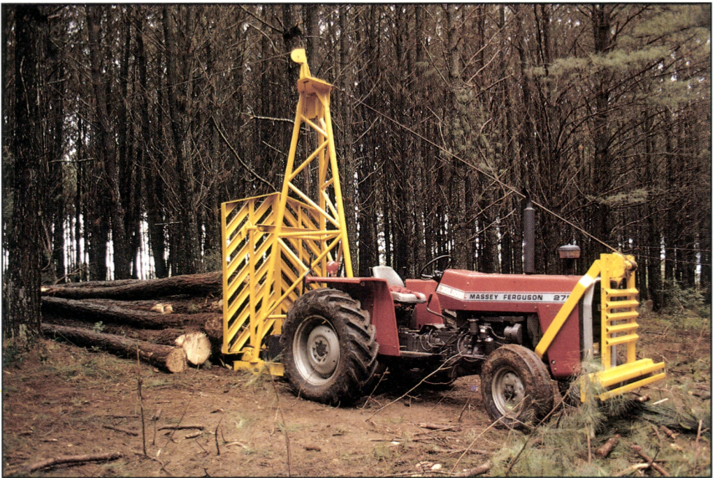
Figure 10. A cable yarding system. Winch with return cable mounted on a Massey Ferguson farm tractor in a Brazilian pine plantation in steep terrain (Photo Jorge Malinovski).
