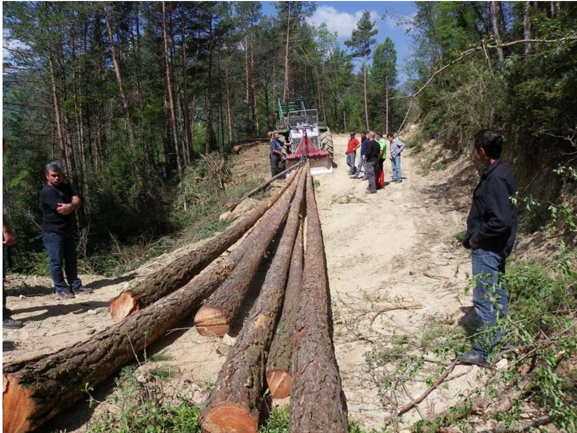
Figure 4: Whole stem yarding with synthetic cable
