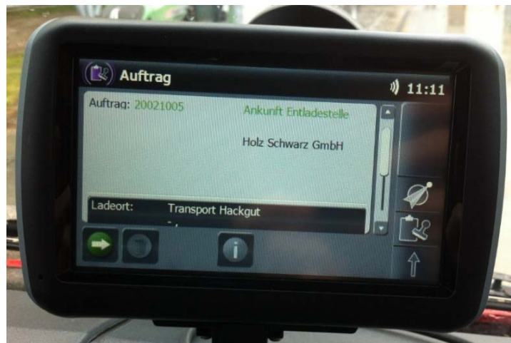
Figure 2 – Hardware (touch display) of the fleet management system used at the entrepreneur Holz Schwarz GmbH. Drivers use this to document working processes and additional information (Poier & Holzleitner).
