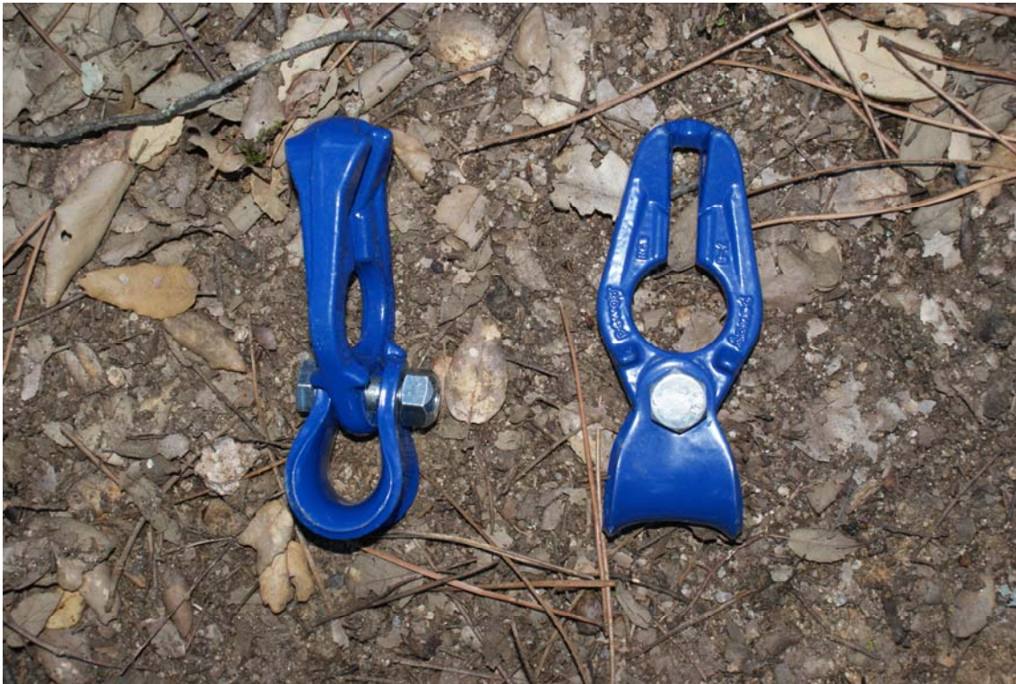
Figure 7: Chokers to be used with synthetic rope
