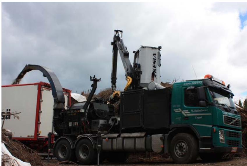
Figure 1 – Chipping non-merchantable roundwood (top) and logging residues (down) with the Kesla C 860 H hybrid chipper during time studies (Photos: Petri Kaksonen/Kesla).
