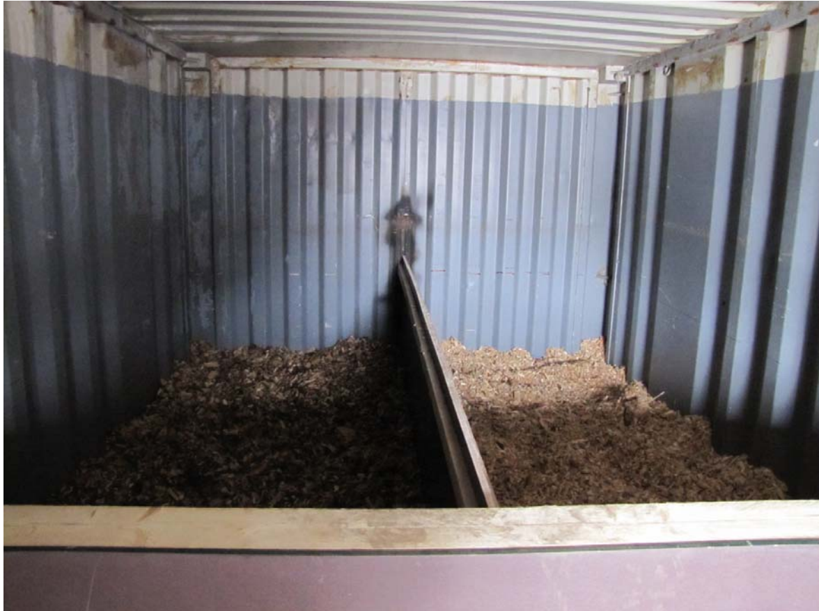
Figure 3. The drying chamber was divided in two boxes so that it was possible to test and demonstrate the drying of two different wood chip types.
