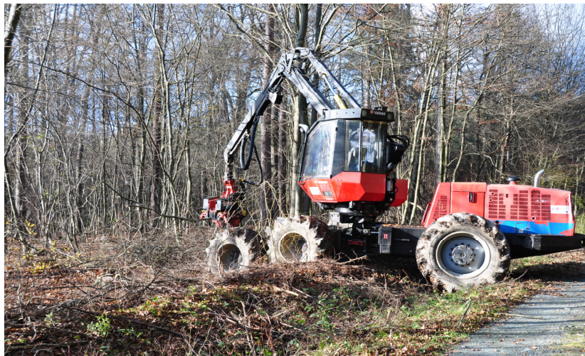
Figure 2 – The energy wood harvesting head EF28 (left) and the base machine Komatsu 911 harvester (right). Picture: Holzleitner, F.
