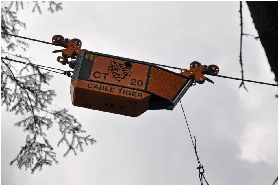
Figure 5: One of the newest small-scale motorized carriage
