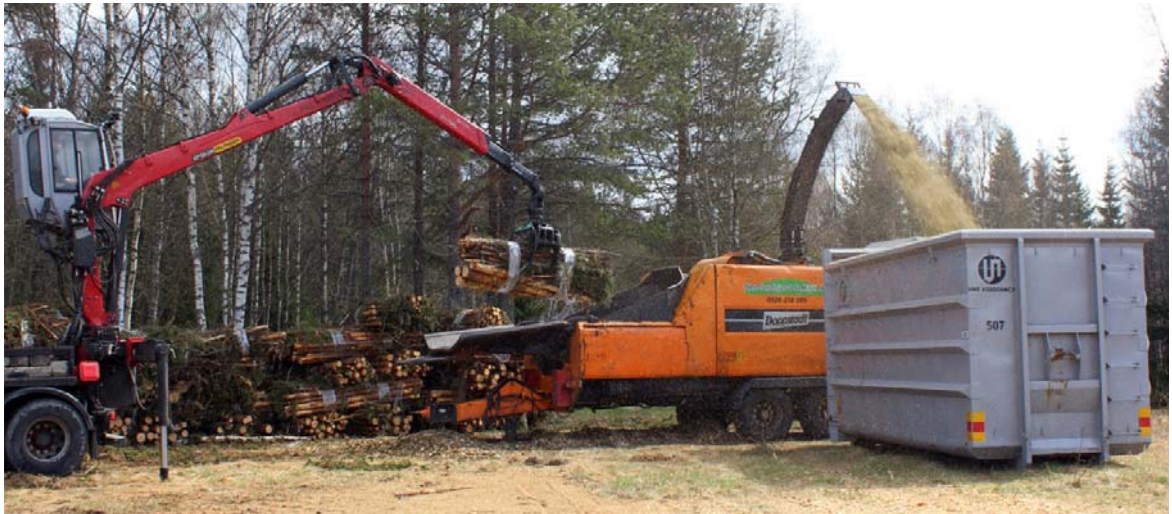
Figure 9. Chipping of bundles with a Doppstadt DH-910 drum chipper.
