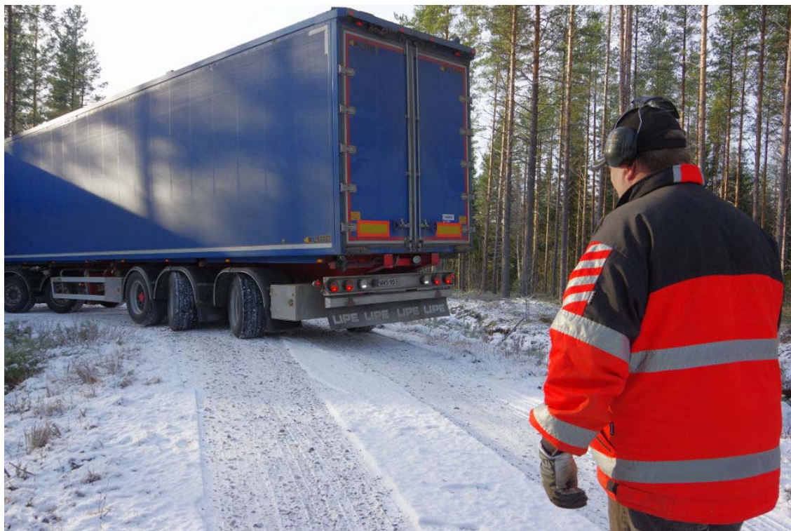
Figure 7. The truck is reversing and the chipper operator is manually steering the rear axles of the trailer by using the remote control (Figure 6). The communication between the truck driver and chipper operator was performed by mobile phone.
