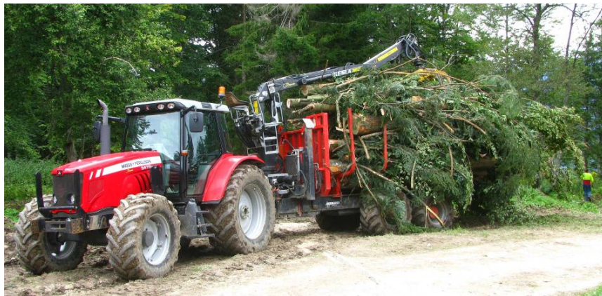
Figure 6. The farm tractor-forestry trailer unit with a load of forest residues.
