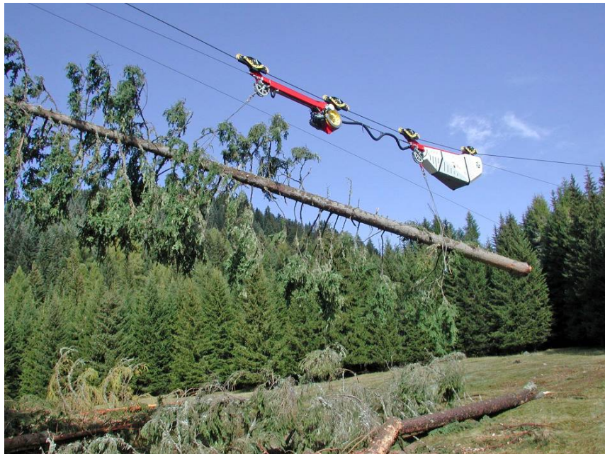
Figure 4: Full suspension achieved with a motorized twin-carriage
