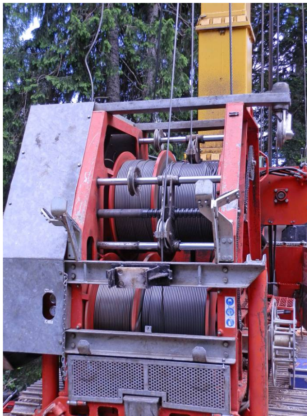
Figure 7: Power is sourced from the yarder winches, not from an on-board engine
