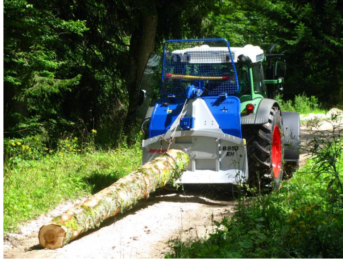
Figure 3. Winch equipped with synthetic cable mounted on a farm tractor.
