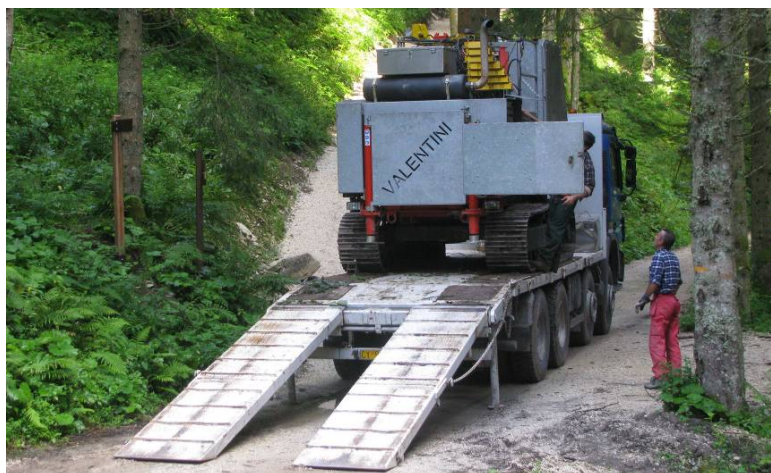
Figure 4. The compact V 600 track-mounted yarder being loaded on its transport.
