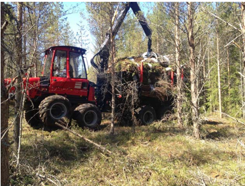
Figure 6. Forwarding of bundles with a Komatsu Forest 865 forwarder equipped with a slash grapple (E36) and a crane-scale system (Intelweigh XW 50PS).
