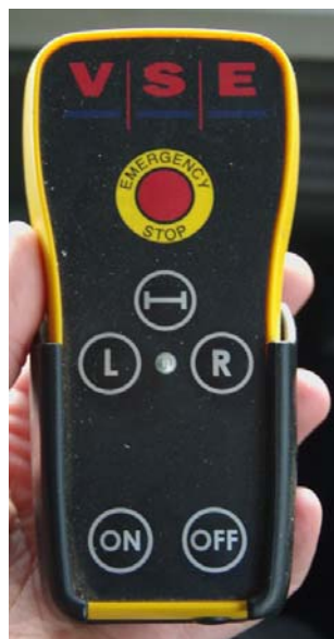
Figure 5. Manual remote control of the ETS: It is possible to control manually the angles of the rearmost axles of the trailer. The mobile remote control enables second person to steer the rear of the trailer around a blind corner.
