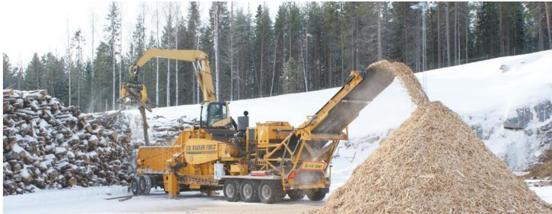
Figure 5. Grinding on a satellite terminal.
