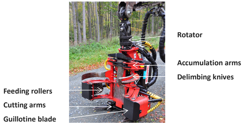
Figure 1: EF 28 head main parts.
