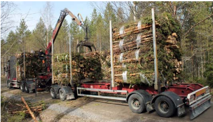
Figure 8. Bundles are loaded on a conventional timber truck.
