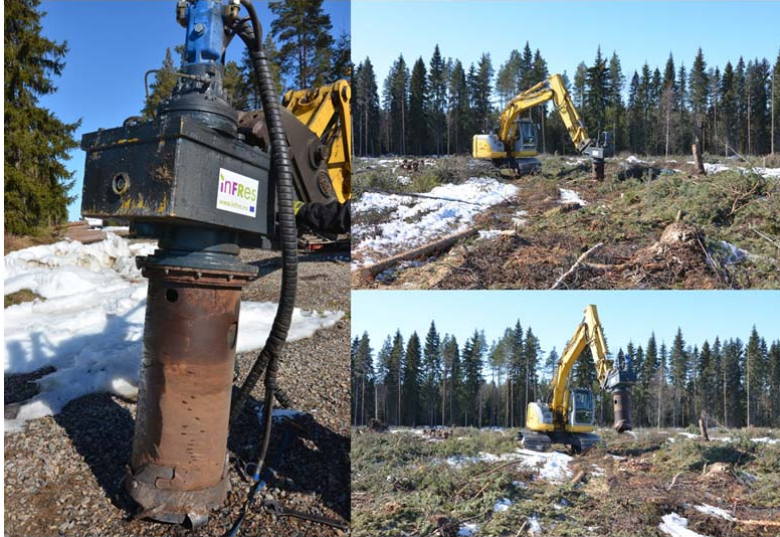
Figure 1. Ellettari stump drill mounted on New Holland excavator in Finnish sites.
