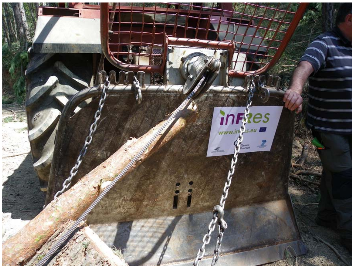
Figure 3: Steel cable winch detail
