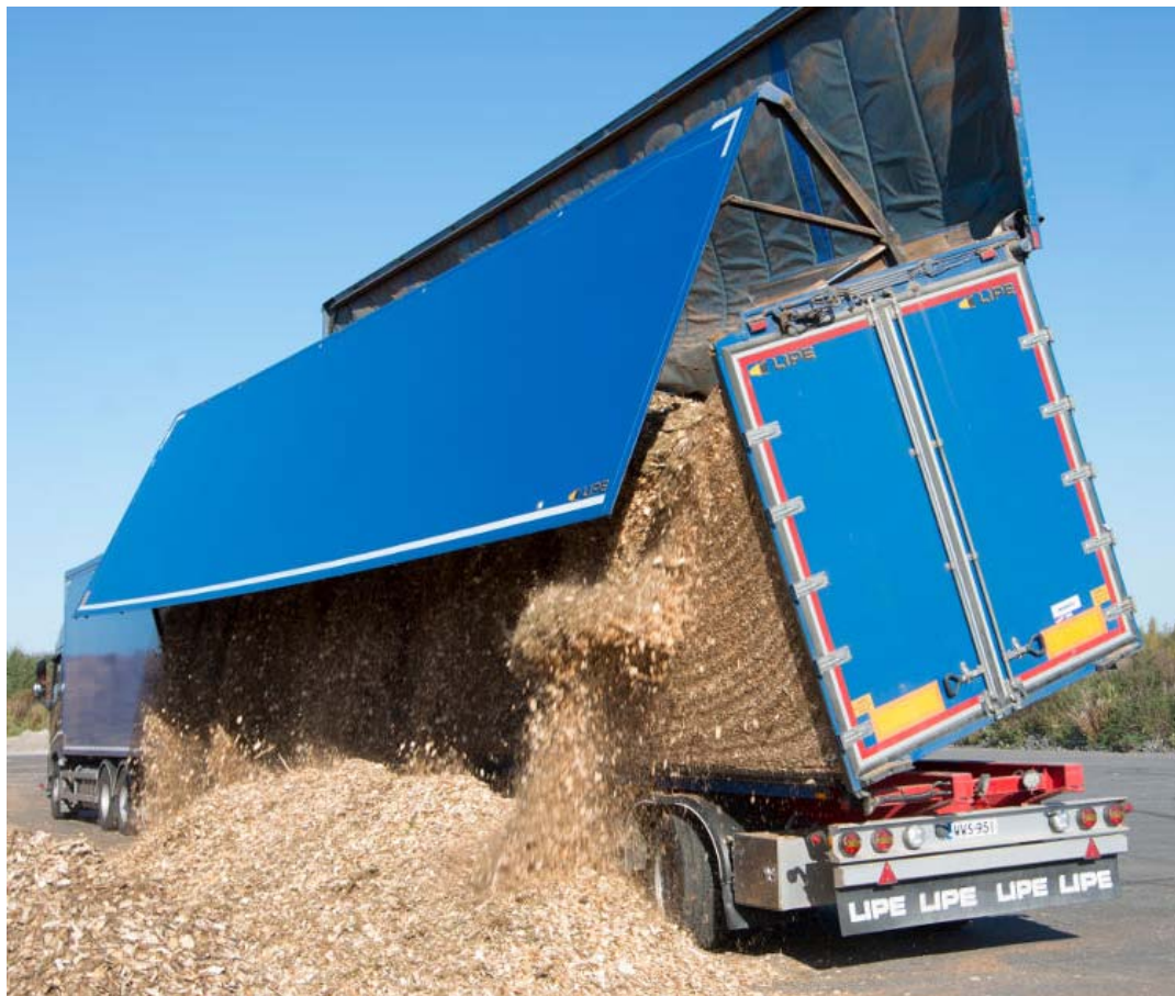
Figure 9. During the unloading the driver steers the rear axles of the trailer away from the chips.
