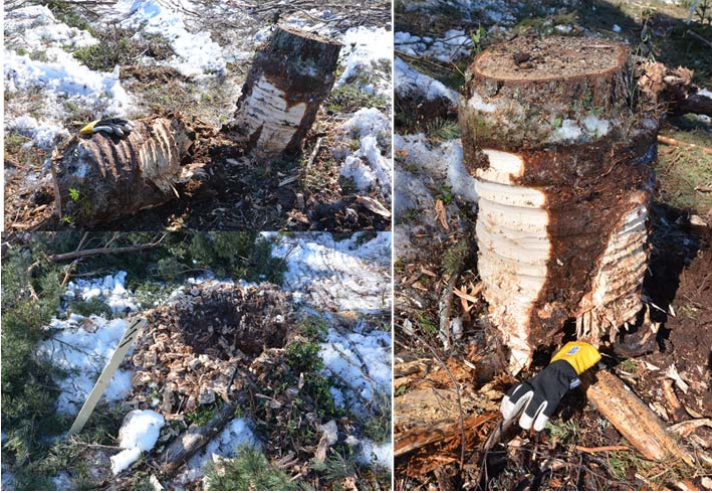
Figure 4. Pine stumps extracted with the Ellettari stump drill.
