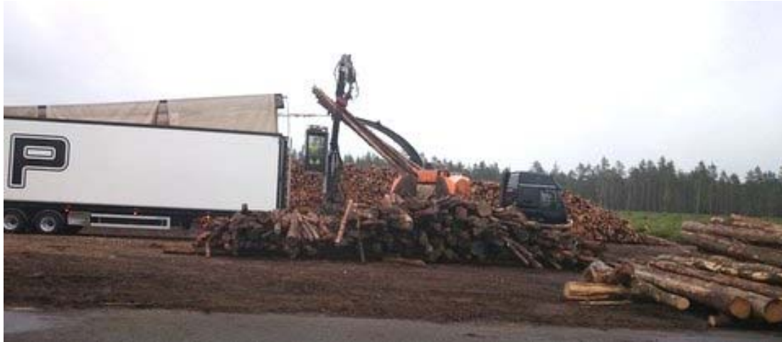
Figure 5. Several manufacturers of equipment demonstrated there products at Stockaryd. Here a chipper-truck, built by OP System, chipping into the trailer.
