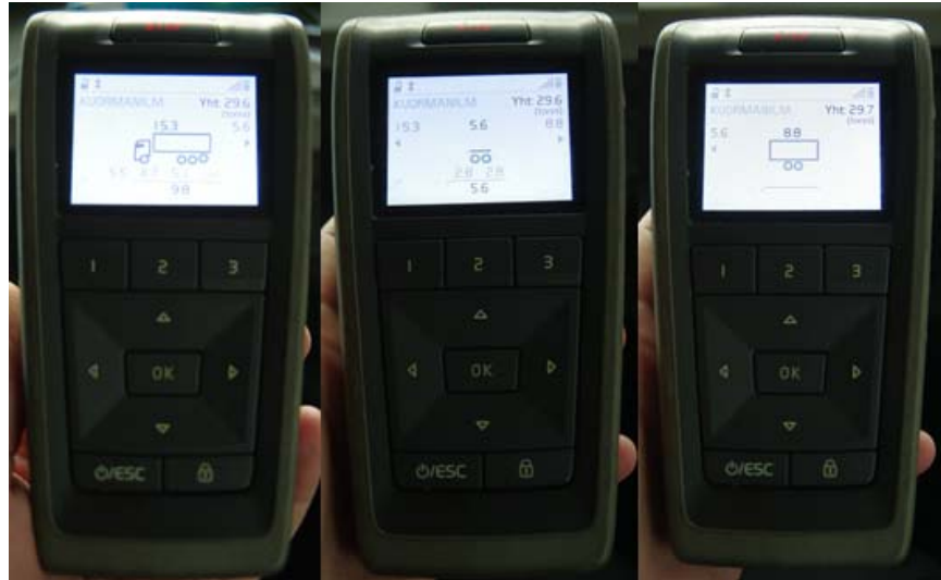
Figure 6. Axle load monitoring device.
