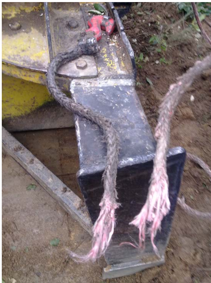
Figure 5: Breakage at the end edge of the synthetic rope
