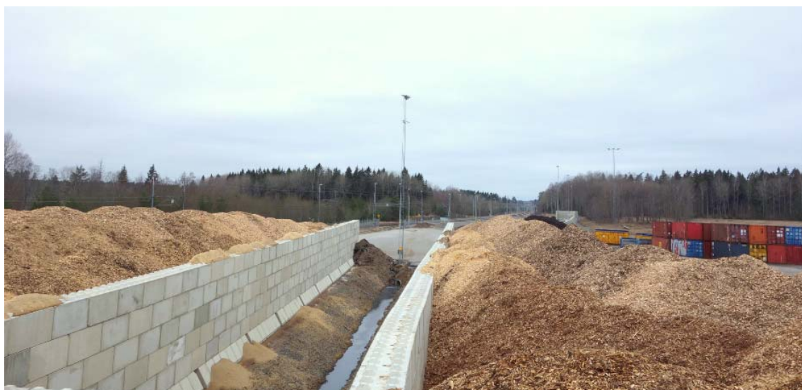
Figure 2. Building blocks separating material from a ditch increases the terminals storing capacity.
