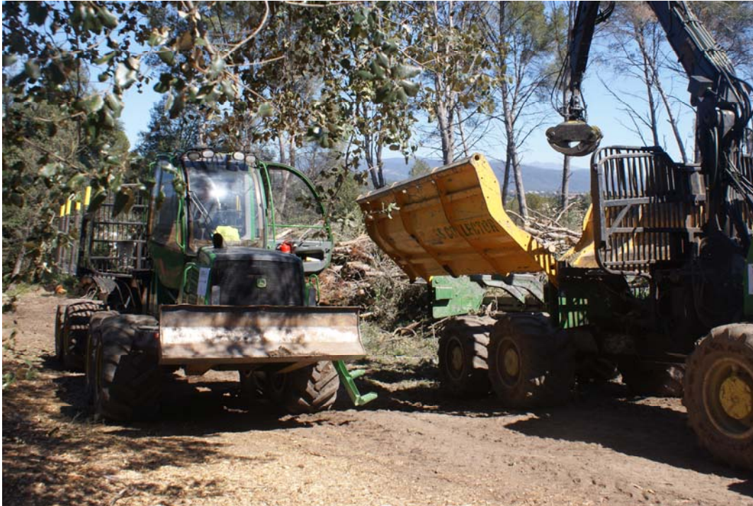
Figure 1: John Deere 1510 on the left and Press Collector on John Deere 1710 on the right.
