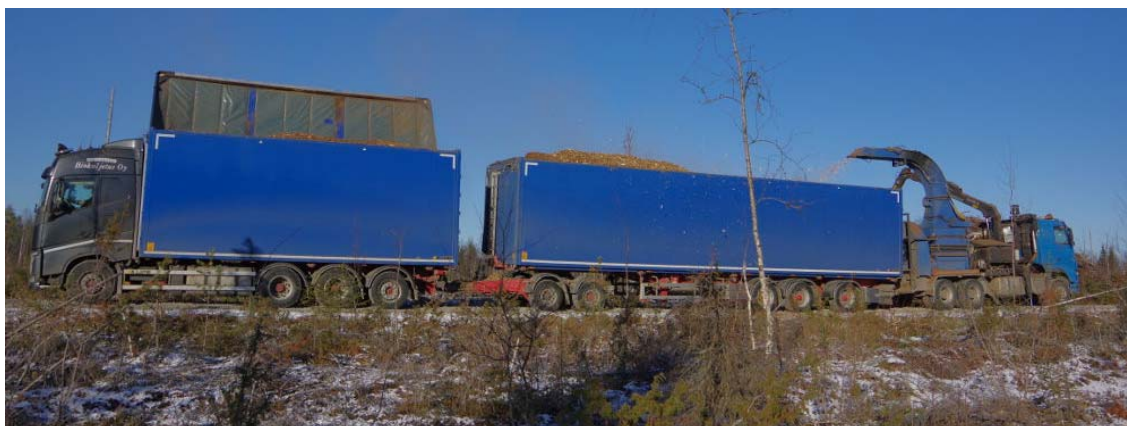
Figure 1. The nine axle multipurpose chip truck constructed by Konepaja Antti Ranta, here loaded directly with a chipper from the rear. Picture: Sami Lamminen, Luke
