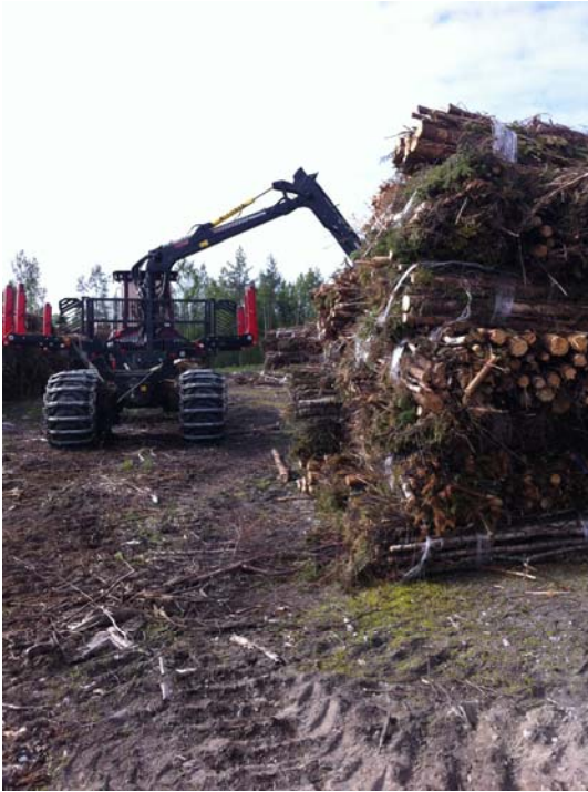
Figure 7. Building of a storage pile. Bundles are laid in cross sections for higher wind penetration.
