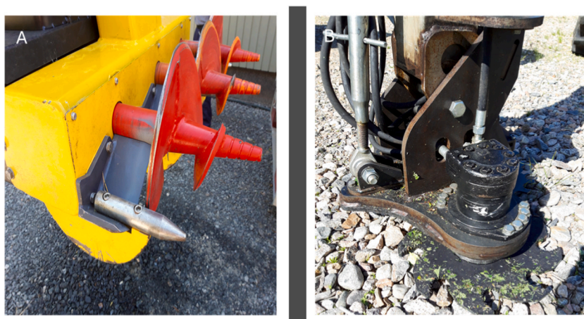
Fig. 2. Cleaning and spreading head options investigated in this study. (A) In the Cutlink head, red rotating spire screws force the stems of seedlings against fixed grey blades, and the inoculum medium of Chondrostereum purpureum is sprayed from the underside of the blades. Yellow side walls prevent inoculum from spreading further from the locations it has been spread. (B) In the Vihtoja head, cogged collecting blades gather the stems of saplings for the fixed cutting blade, and the spreading nozzles spray the inoculum medium on the upper surface of the collecting blades. Photos: Leena Hamberg.
