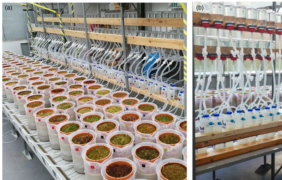
FIGURE 1 (a) Mesocosms in the water table (WT) control cylinders constructed following the design outlined in Nijp et al. (2014) with (b) WLD of 20 cm introduced by lowering the position of control reservoirs. Mesocosms were organized into four rows containing a complete set of experimental variables (treatment \times species \times origin peatland type \times WT history) and four complete blocks along the length of the table.
