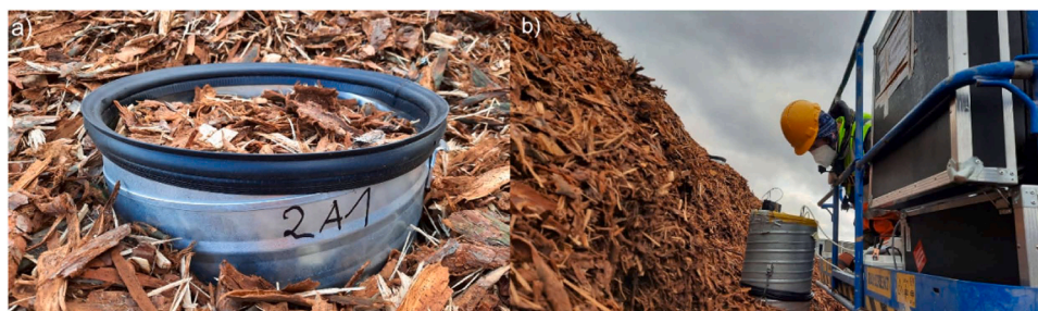
Fig. 3. The collars for the chamber measurements were permanently buried in the bark stockpiles (a). A flux chamber was placed on top of the collars, with a closed circulation between the chamber and gas analyser during the measurement (b). The system was operated from a crane to avoid disturbance and compression (Photos: Luke/Alm Jukka).
