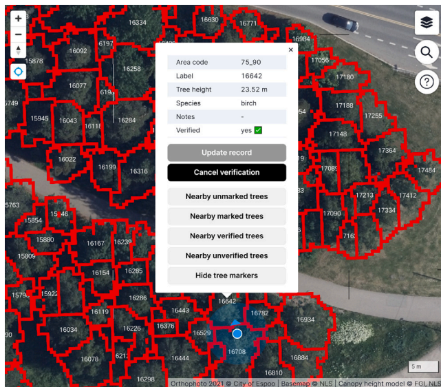
Fig. 4. Screenshot of the crowdsourcing application used to collect ground-truth species data. In this example, the application shows a true orthophoto map, segment boundaries (red lines), the surveyor's location (blue circle) based on GNSS positioning, and the information of the nearest segment together with possible actions for the surveyor. The true orthophoto map in the background was obtained from the City of Espoo (2024) .
