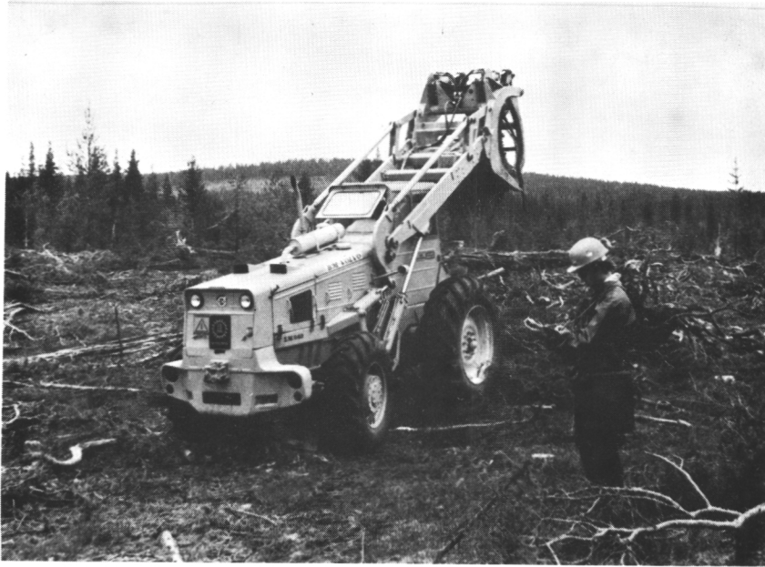
Extracting of stump-root systems by wheel loader
