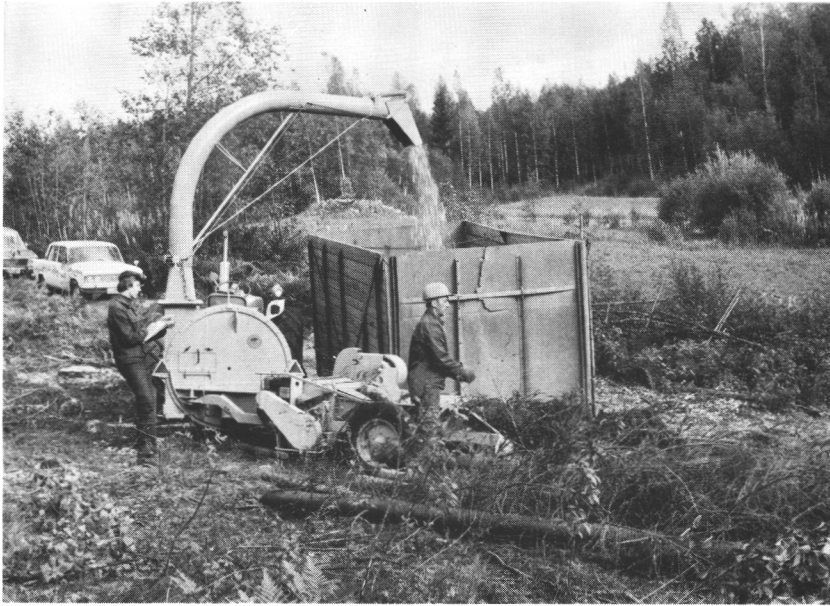
Chipping of complete small-sized spruce trees
