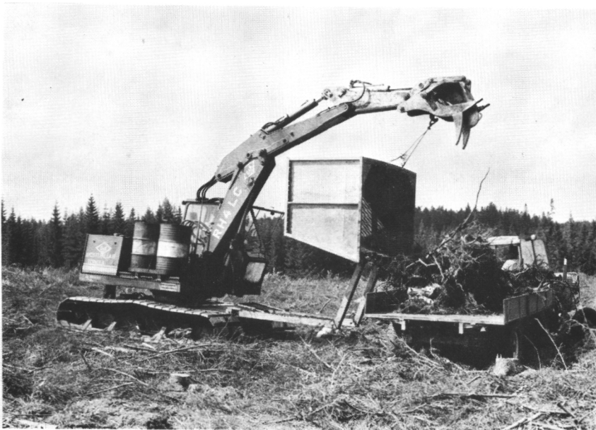
Harvesting of stump and root wood by the Pallari Stumparvester
