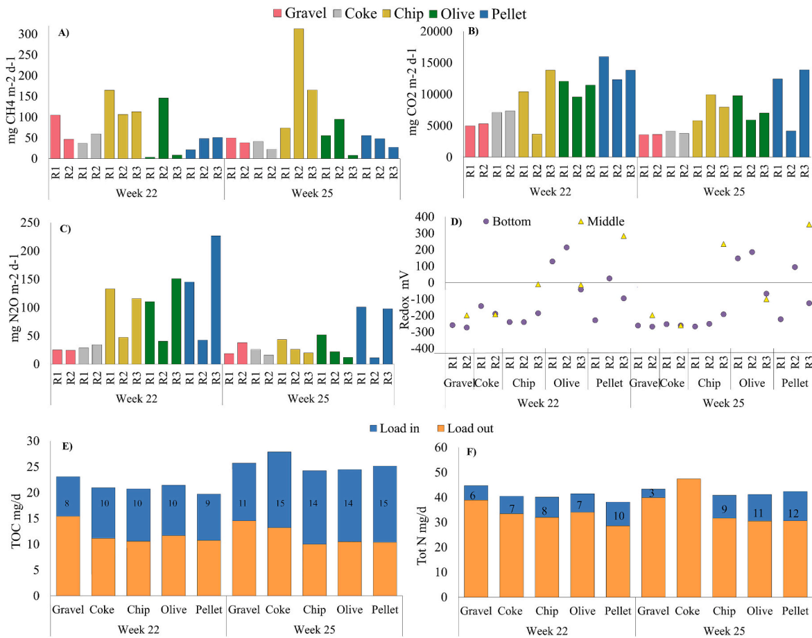
Fig. 3. Gas emissions for each material and replicated system (A-C), redox measurements during gas sampling days (D), and inflow and outflow daily load with load removal provided as values inside the bars (E-F). Replicate columns of the same material are referred to as R1, R2, or R3.
