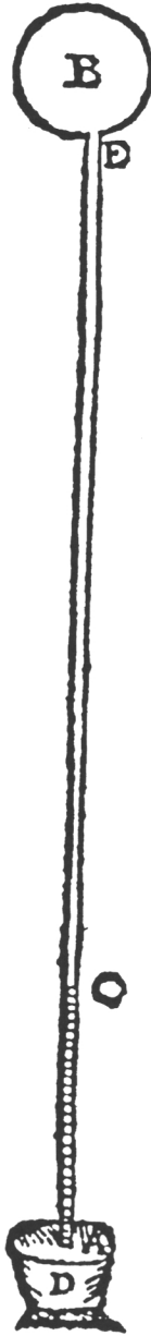
Figure 5. The first published drawing of a thermometer (Biancani 1620 cit. Middleton 1966).
