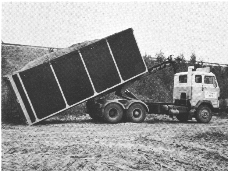
Figure 30. The Multilift ML-14 pallet system in connection with terrain chipping by a TT 1000 F.
