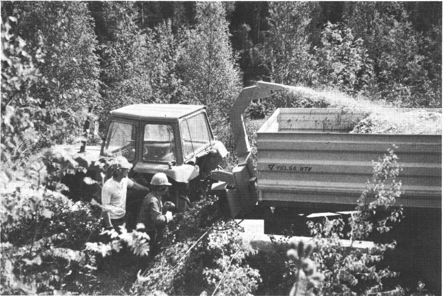
Figure 21. The AST whole-tree chipper attached to the three-point lift linkage of a farm tractor. Manual feeding.
