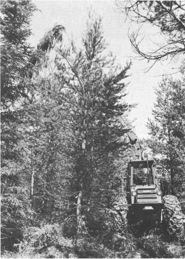
Figure 12. The Marttiini slide boom mounted on a Valmet 872 forwarder (photo Valmet Oy).
