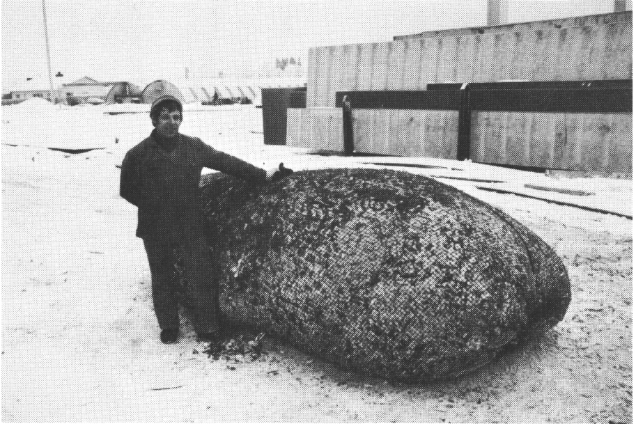
Figure 20. A nylon mesh sack system for transporting whole-tree chips is under development.
