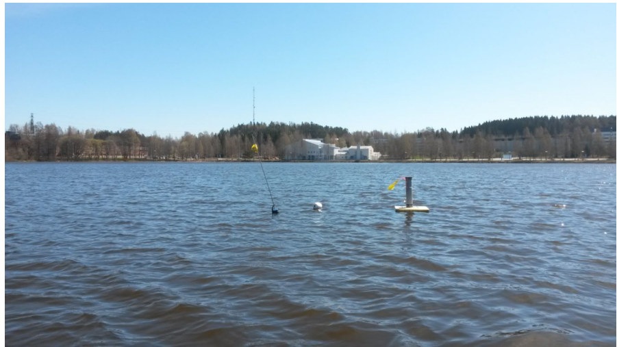
Fig. 2 Online trap in Savilahti bay basin at a depth of 6 m under the flag sign. Anchored float behind flag sign is the base station for the online trap, which sends measurements to the Internet over a mobile network
