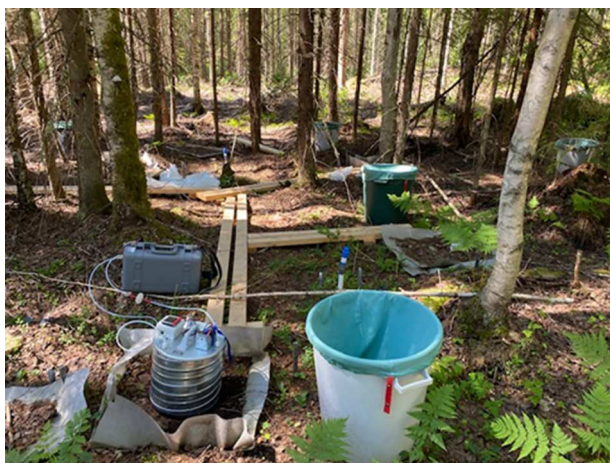
Figure 1. Heterotrophic soil respiration measurement setup using a LI-COR 7810 gas analyzer connected to a closed dynamic chamber. The setup also includes a foliage litter collection container.
