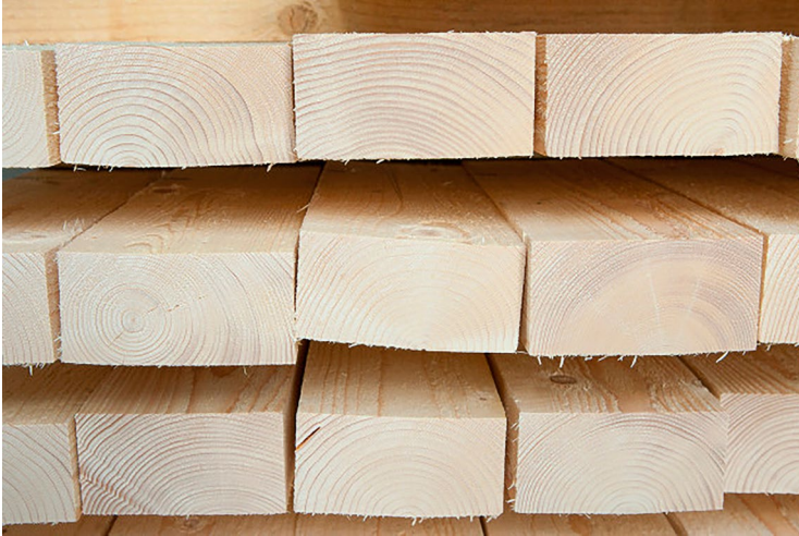
Fig. 9.8 Severe twist in the board in the center among boards with little or no twist. Photo Erkki Oksanen/Luke
