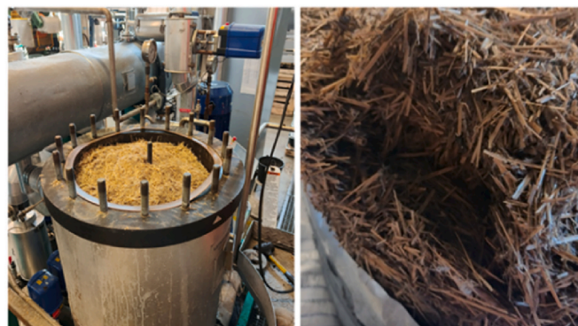
Fig. 1. The extraction reactor of PHWE filled with common reed (left) and wet extracted reed (right).
