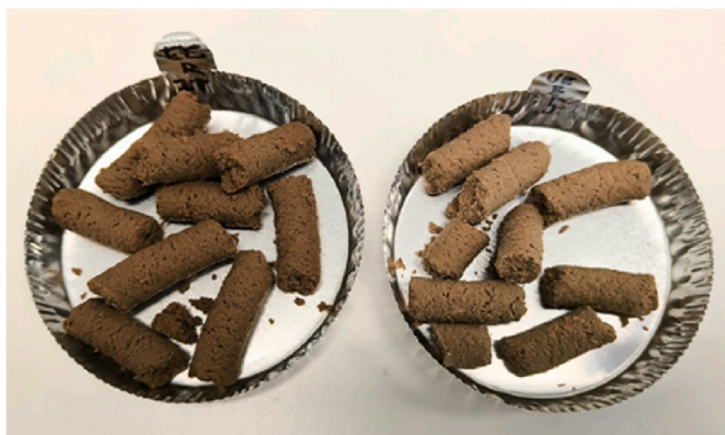
Fig. 2. Reeds after extrusion. Extracted reed with darker color is on the left and untreated on the right.
