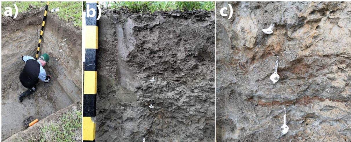
Figure 9. The Maaninka 05 pedon (Keskilohko field plot). The sandy loam and silt loam pedon had a grayish colour (a and b) but there was substantial mottling of brown redox concentrations and gray redox depletions (c). Photos by Mari Rätty (Luke).
