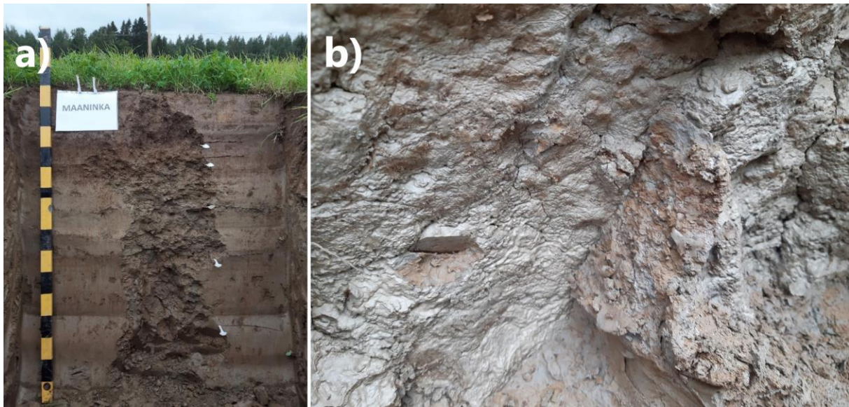
Figure 19. The Maaninka 14 pedon; Anttila 1. As usual, the soil had brownish colours in the upper horizons and grayish colours deeper in the soil profile (a). The desiccation cracks in the subsoil were covered with a continuous gray layer of illuvial material transported from above (b). Photos by Mari Rätty (Luke).
