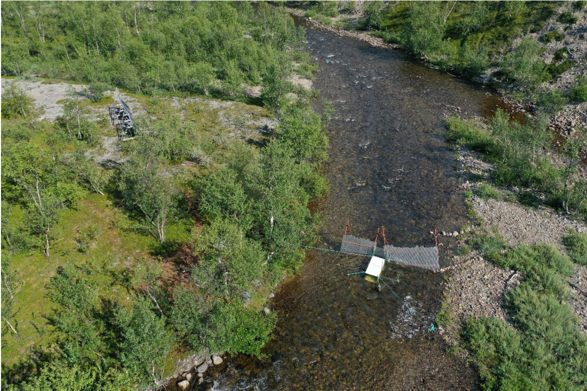
Figure 6. Simsonar FC stereo camera system installed to the River Gálddašjohka/Kalddasjoki in 2024. The white box in the middle of the river is the camera tunnel unit. Guiding fences goes from the tunnel unit downstream to both shores. Data recording and solar power systems are situated on the shore (left hand side). Photo: Mikko Kytökorpi.
