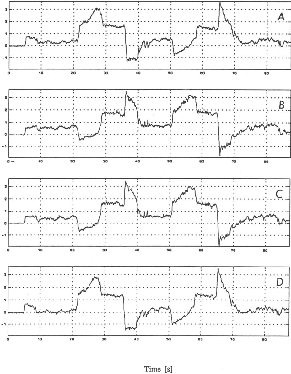
Fig 8. Torque while driving in a S-kurve without load on asphalt with 8-WD. A: Left front bogie B: Right front bogie. C: Left rear bogie. D: Right rear bogie.
