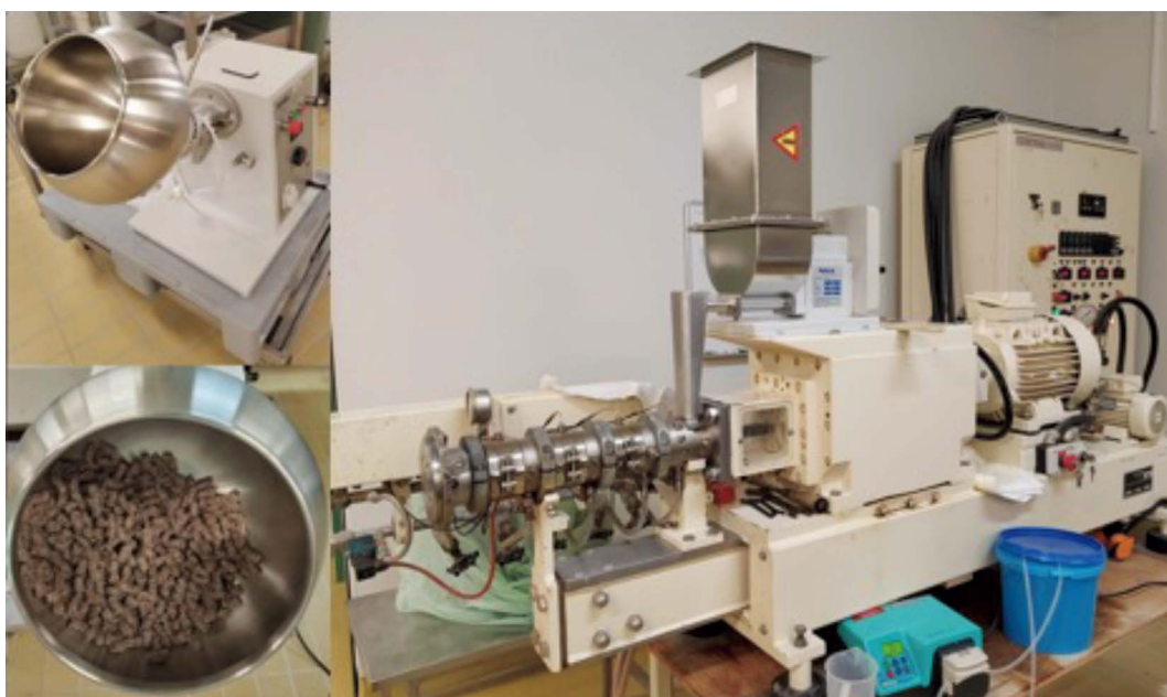
Figure 1. Erweka AR 403 coating drum and Clextral BP10 twin-screw extruder.
