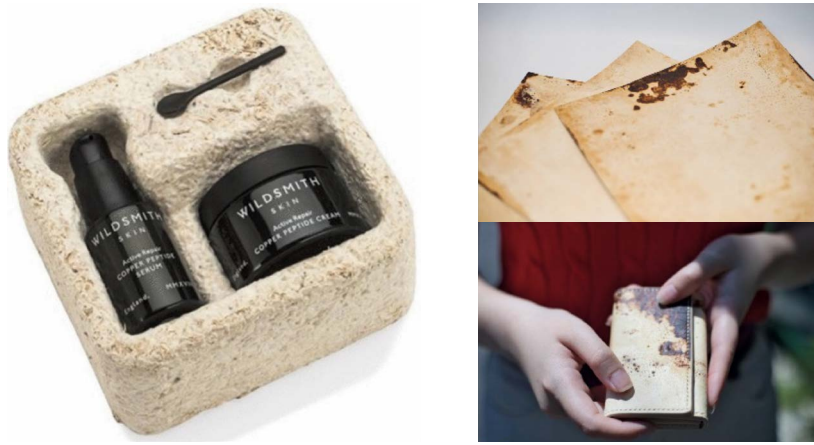
Figure 2 Mycelium-based composite for packaging material (S. Vandelook et al. 2021, ©Ecovative) and business card holder made of mushroom leather (©mushco).
