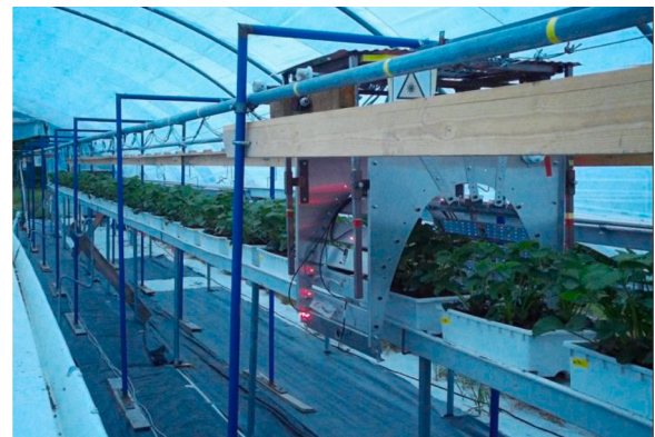
Fig. 2. LED-based UV-exposure equipment developed for research purposes in Suonenjoki, Finland.
