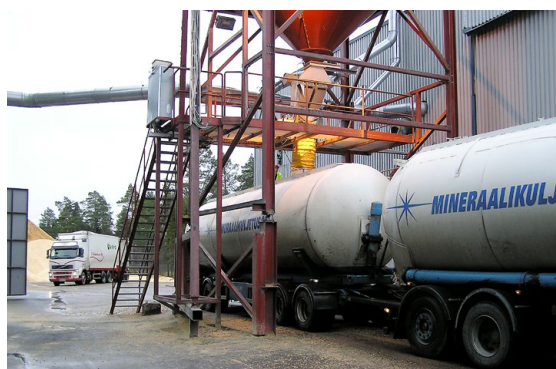
Figure 21.8. Loading pellet to pneumatic truck from silo and warehouse (©Metla).
