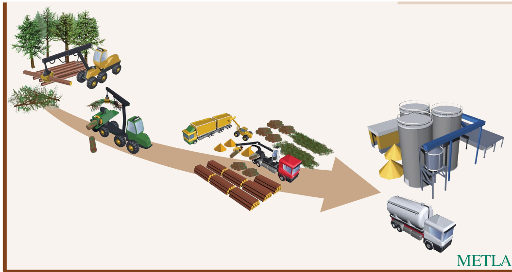
Figure 21.3. Logging residues from forests to pellet production with bundling method
