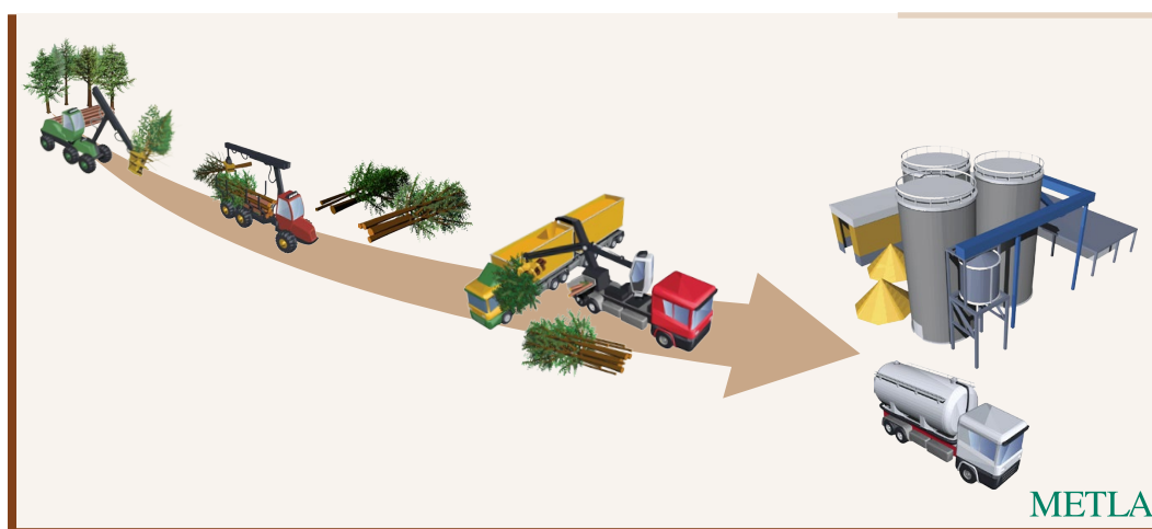
Figure 21.7. Mechanized harvesting of whole trees, roadside chipping and delivery of chips from the roadside to the pellet plant.
