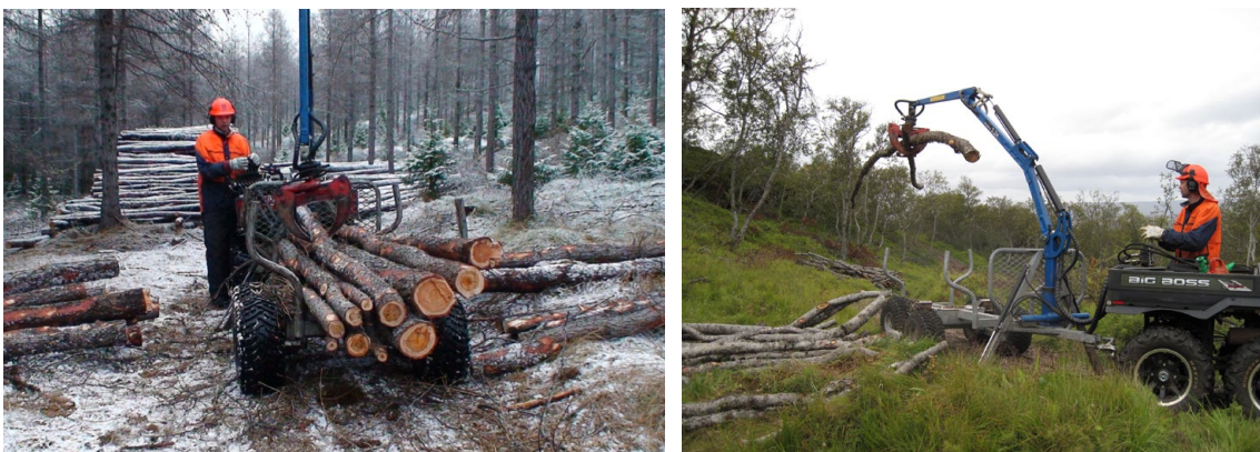
Figure 21.5. Small scale forwarding with ATV after motor manual felling in Iceland. (© Robert Prinz)
