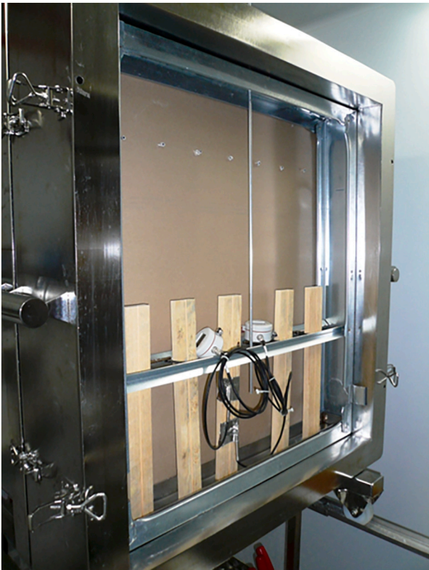
Fig. 2. Test wall structure opened. At the beginning of the test, five wooden laths were placed vertically in a steel basin inside the wall structure to which water was added at the beginning of the test. There was visible mold growth on the surface of the wood in the picture. The variation in the relative humidity and temperature of the wood material was measured with a surface sensor taped to the surface of the wood.
