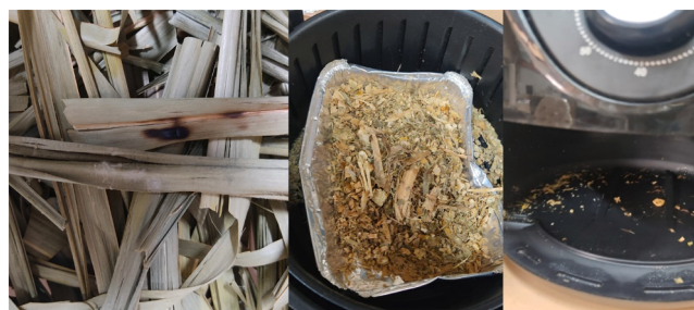
Fig. 5. Examples of blunders caused by the use of an air-fryer equipment during the partial dehydration process of forage samples.
