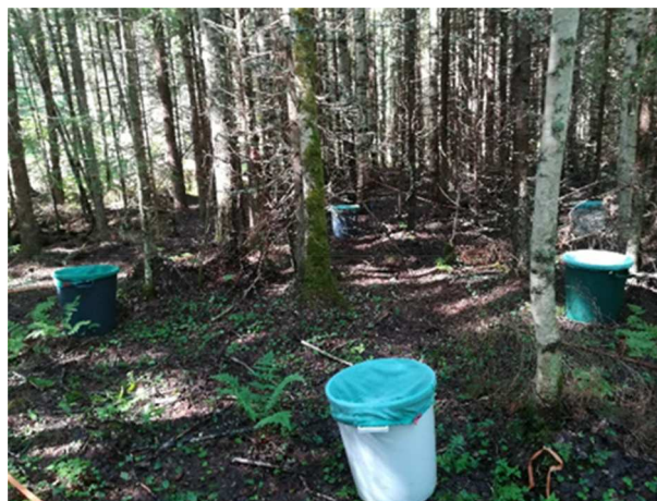
Figure 1. Foliage biomass collectors installed in a drained peatland forest for litterfall measurement.
