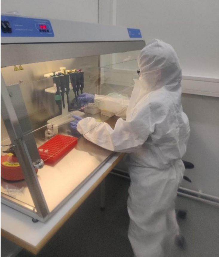
Figure 3. eDNA laboratory dedicated for reagent pipetting in Luke, Jokioinen. As eDNA is easily contaminated, eDNA laboratories (DNA-free) are isolated from other laboratories and contaminations are prevented by wearing fully covering overalls. UV light, ethanol and chlorine are used to sterilize rooms and PCR cabins.
