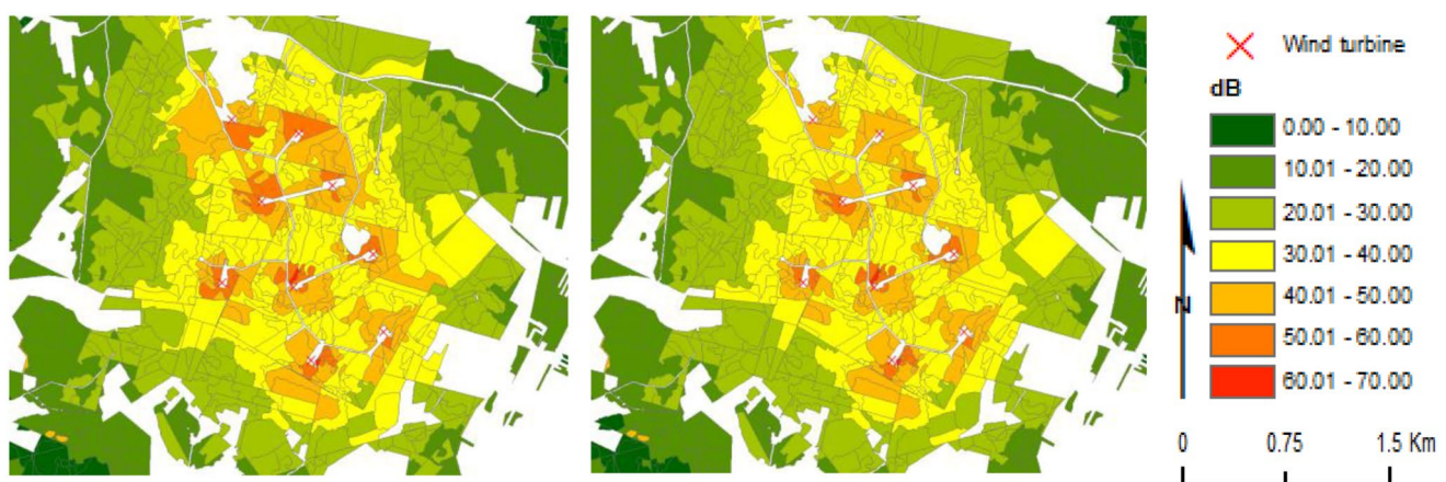
Fig. 3 Turbine noise in the wind turbine neighbourhood at the third 10-year period. Noise over 40 dB = colours from orange to red. Even-aged forest management and even-flow of timber, linear-shaped sub-
