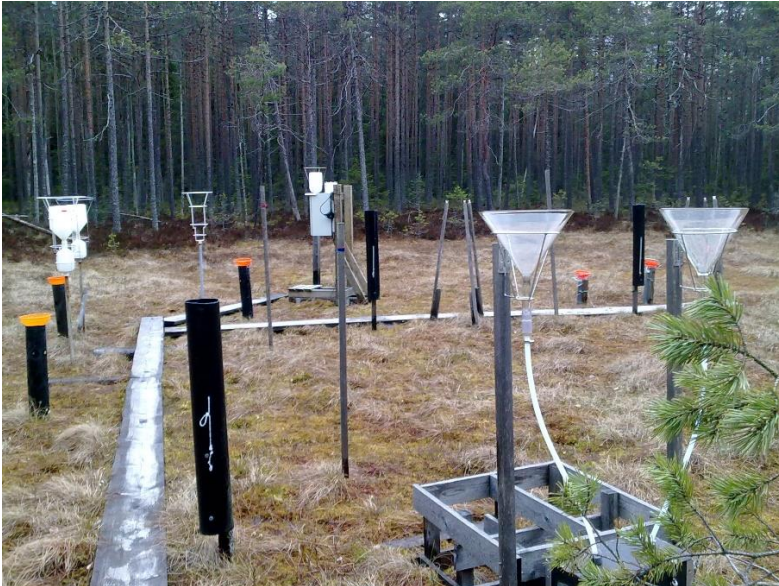
Figure 3. Collection of bulk deposition samples. White funnels are official collectors of Finnish Meteorological Institute, orange funnels are set by Natural Resources Institute Finland (Luke).
