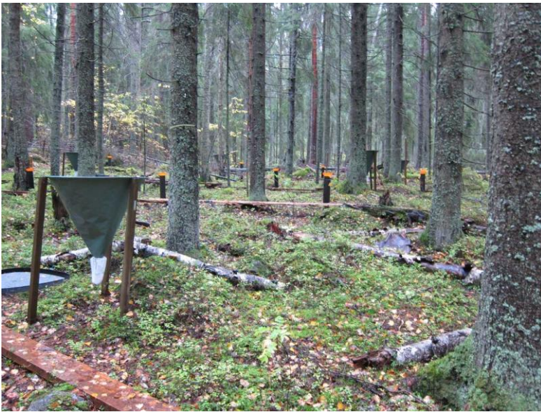
Figure 4. Throughfall (orange funnel) and litterfall collectors (green funnels) in Valkea-Kotinen. Photo: Liisa Ukonmaanaho.
