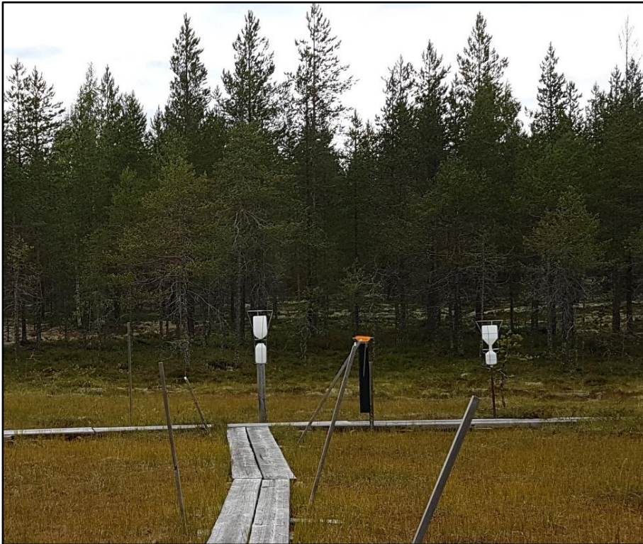
Figure 3. Collection of bulk deposition samples. White funnels are official collectors of Finnish Meteorological Institute (right) and Finnish Environment Institute (left), orange funnels are set by Natural Resources Institute Finland (Luke).
