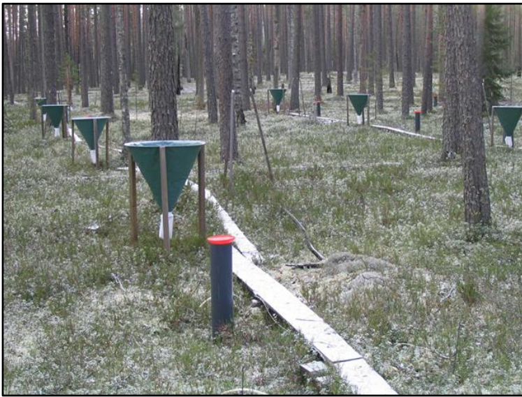
Figure 4. Throughfall (orange funnel) and litterfall collectors (green funnels) in L. Iso Hietajärvi catchment.
