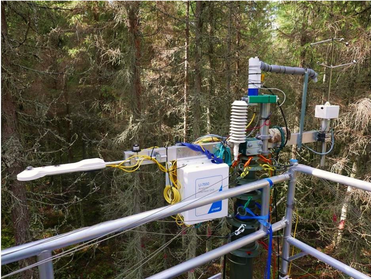
Figure 6. On the right sonic anemometer. Air is sucked via heated and insulated tube to the sensor head of the CO 2 -H 2 O analyzer. The LI-COR electronic box and radiation shield in the middle and radiation sensors on the left. Photo: Tuomas Laurila.
