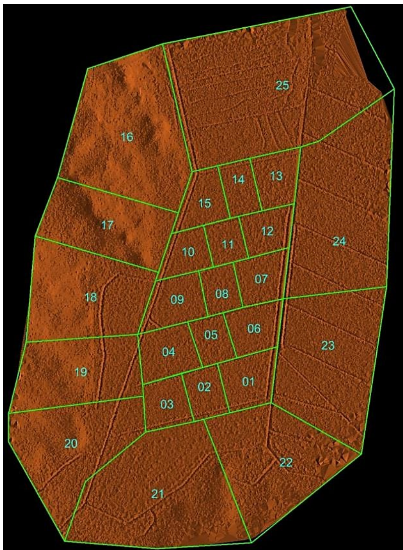
Figure 28. Study site (Paroninkorpi) was divided to 25 blocks for aerial laser scanning with Riegl Ricopter and Riegl VUX-1UAV scanner.
