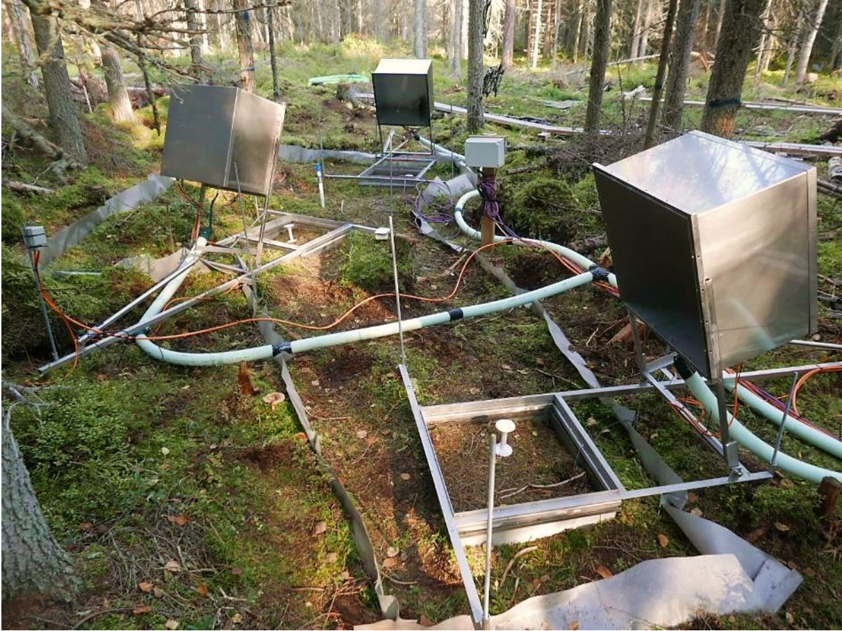
Figure 14. Three opaque chambers at the trenching experiment close to the micromet flux tower. Photo: Tuomas Laurila.
