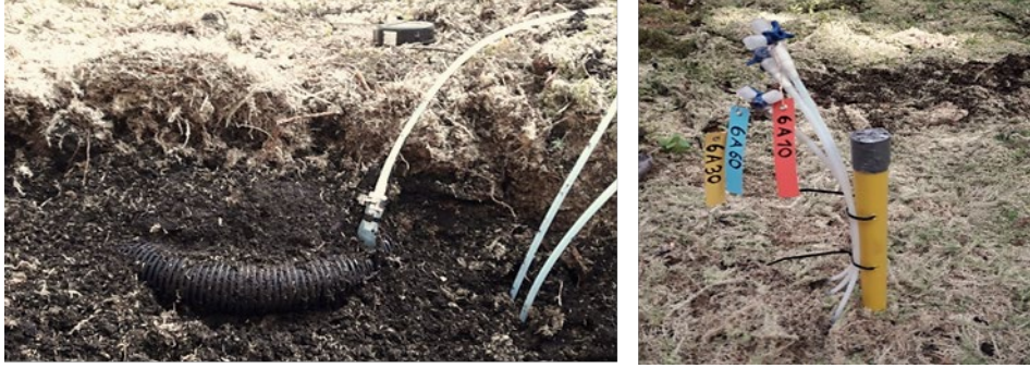
Figure 31. Gas collector unit belowground (left) and setup with PTFE tubings and valves aboveground. Photos: Mitro Müller.
