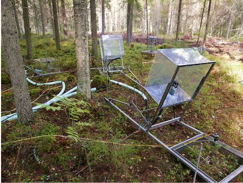
Figure 12. In 2019, six automated chambers for forest floor greenhouse gas flux measurements were made operational at Ränskälänkorpi site. Photo: Tuomas Laurila.
