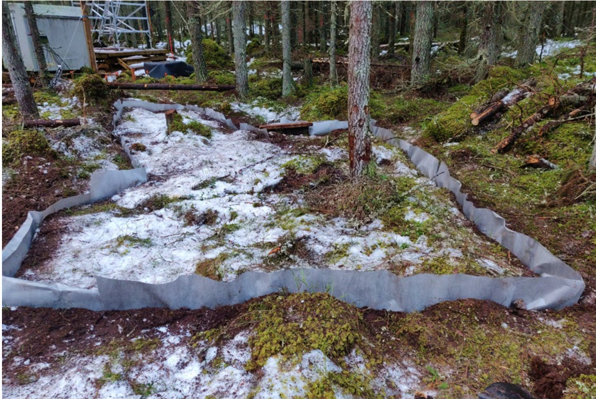
Figure 3. The measurement site of heterotrophic soil respiration ( \text{CO}_2 ) in Ränskälänkorpi close to the Eddy Covariance tower. The root layer of the site was isolated from the surroundings by inserting a root exclusion fabric vertically into the soil. The trunk inside the measurement site is a dead tree.
