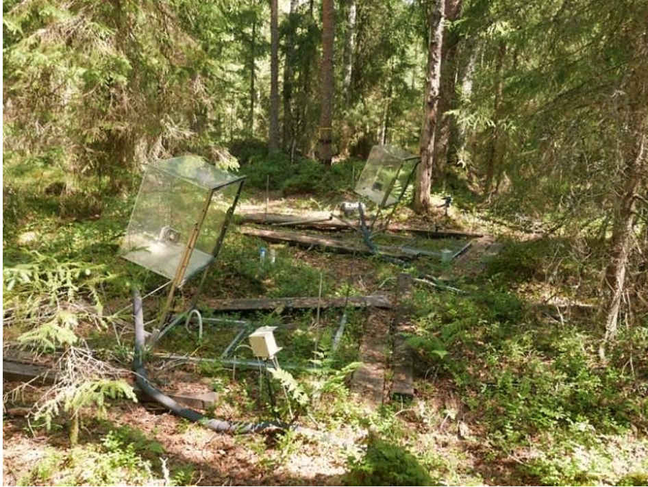
Figure 23. Six automated chambers for forest floor GHG fluxes at Lettosuo. Photo: Tuomas Laurila.
