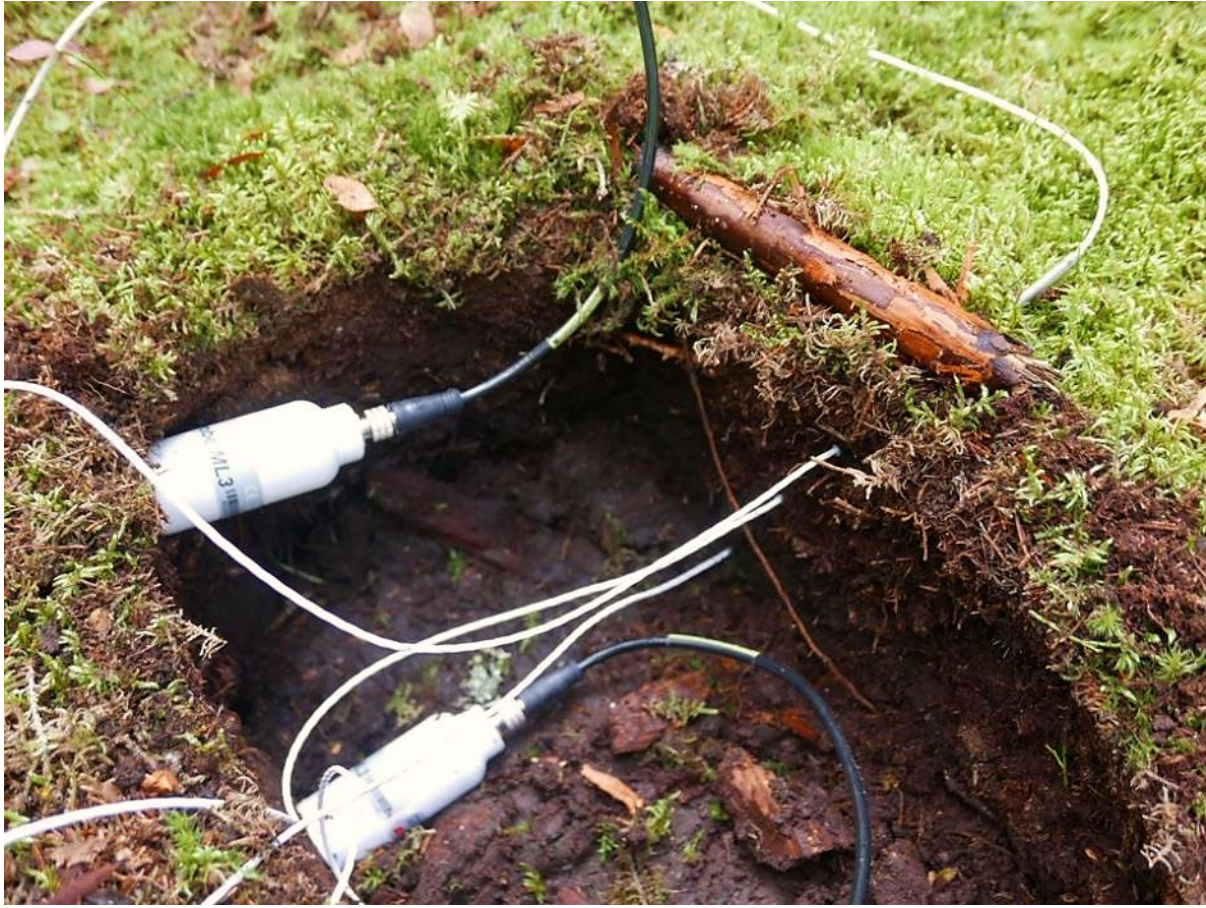
Figure 16. Soil temperature and humidity sensors. Photo: Tuomas Laurila.
