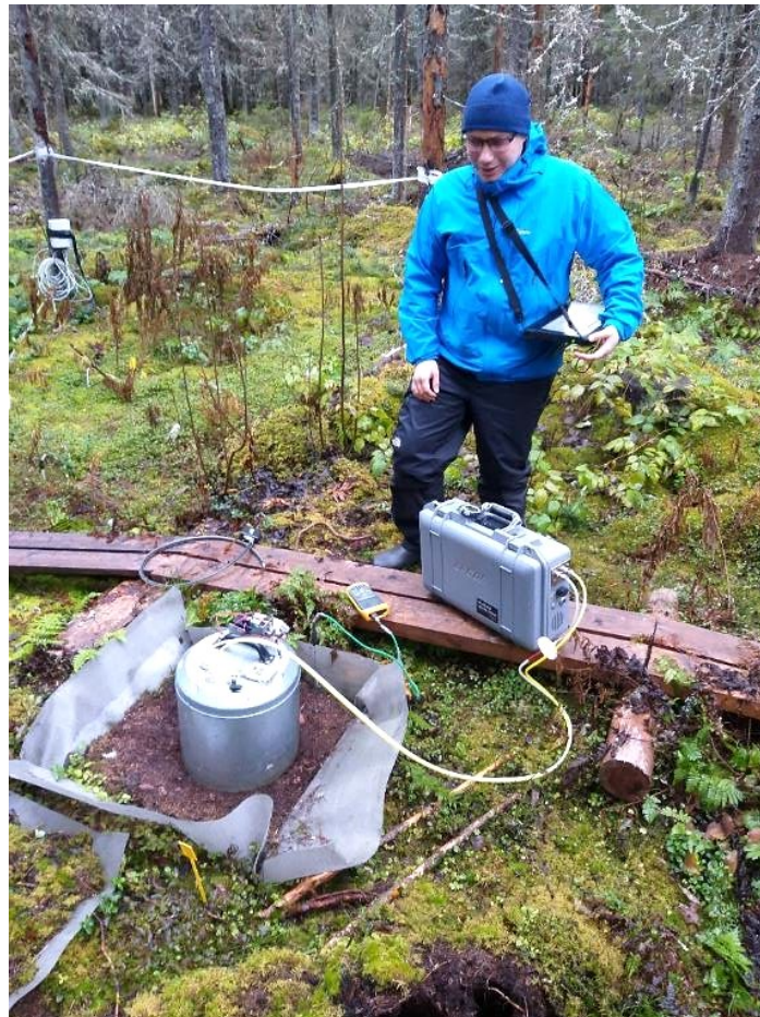
Figure 30. Greenhouse gas (CO 2 and CH 4 ) measurements on Paroninkorpi site in October 2020 by Petri Salovaara with chamber and gas analyser LI-7810 (LI-COR Inc., Lincoln, NE, USA). In Paroninkorpi site, ongoing measurements of CO 2 , CH 4 , and N 2 O fluxes started in 28.7.2017 and were continued in 2019 and 2020 over the snow free period. Heterotrophic respiration monitoring was appended by 4 new points in 20.5.2020. Photo: Raisa Mäkipää.
