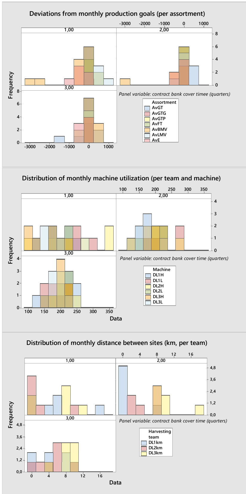
Figure 36. Distribution of monthly production KPIs for three sizes of contract bank (panel variable: 1–3 quarters). Deviations from monthly production goals (above), machine utilization (middle), and distance between harvesting sites (below).
