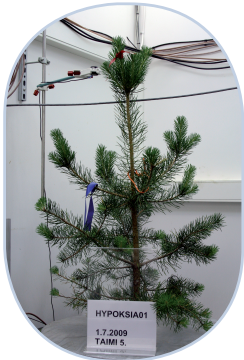
Figure 2. The study was performed in a special type of growth chambers, dasotrons, where air and soil conditions can be controlled independently. Photo: Eija Koljonen.
