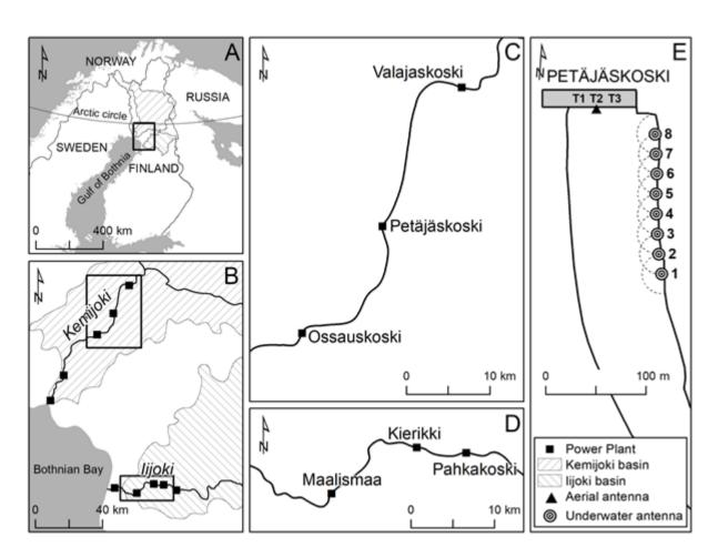
Figure 1. Location of the rivers (A) and location of the hydropower plants (B-D). The frame E in the right shows the setup of the telemetry antennas using the Petäjäskoski power plant as an example.
