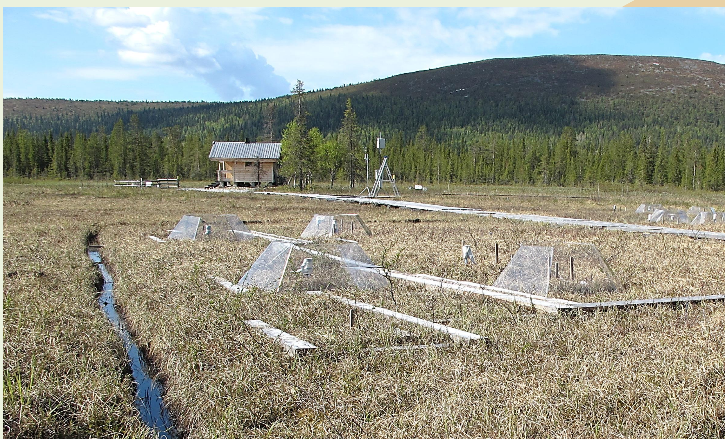
Experimental setup with OTCs and shallow ditches in Lompolojänkkä site
