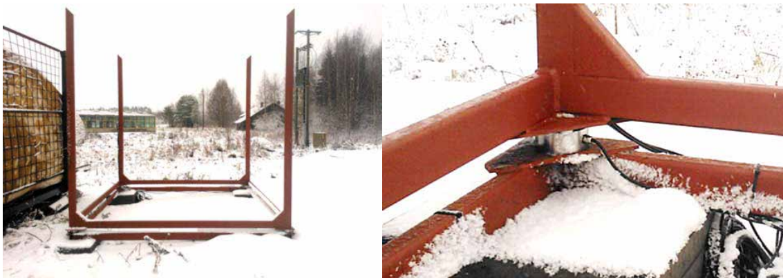
Figure 1. Metal frame (left) and load cells (right) used at the Finland A experiment. Notice the supporting second frame below the load holding frame. Source: Metla.
