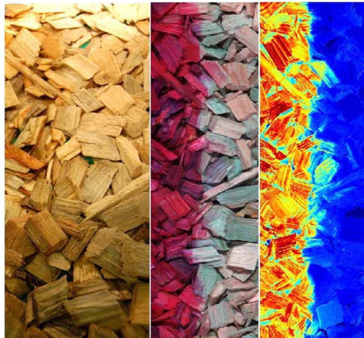
Figure 42. Demonstration of moisture detection with NIR. (Left) A photograph of wood chips on a conveyor belt is displayed. The left half of the particles has been spray-wetted which is seen as a slightly darker colour shade. (Center) The same sample was measured with NIR-CI and the spectral image is displayed here as a pseudo- RGB image using three reflectance values (at 1106, 1945 and 2315 nm) as RGB coordinates. The wet area has relatively higher red component. (Right) The ratio of water/cellulose NIR absorption bands is displayed as intensity image (moisture map). Red/blue colour means high/low moisture level at the corresponding location.
