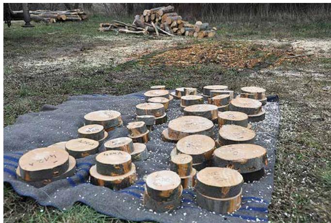
Figure 3: Stem wood sample slices taken at the Austrian drying trials. Source: Gernot Erber.
