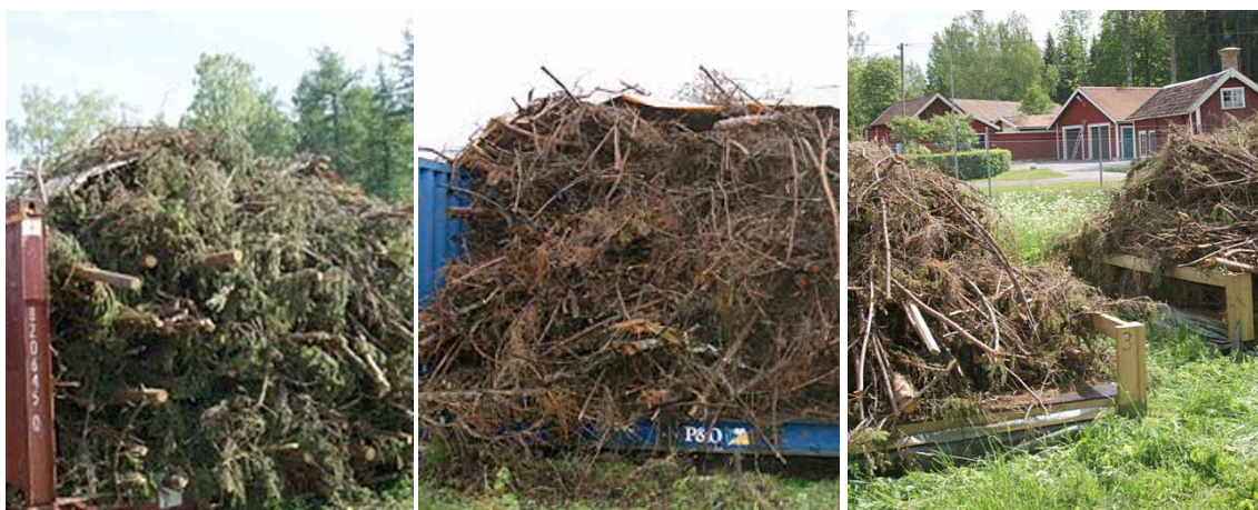
Figure 9. Ship container (left and middle) and self-made wooden platform (right) drying trial types used in Sweden. Source: Lars Wilhelmsson.
