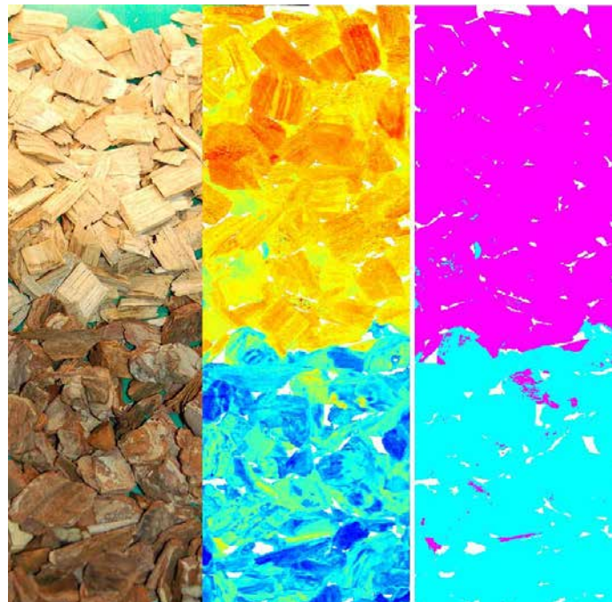
Figure 51. Classification between stem wood and bark particles with NIR-CI. (Left) Photograph was taken of stem-wood chips and bark particles placed on the conveyor belt in separate groups. (Center) Continuous output of a linear classification model (PLS-DA) which was trained on this image. (Right) The pixels are classified into two groups via thresholding the values of the center image.
