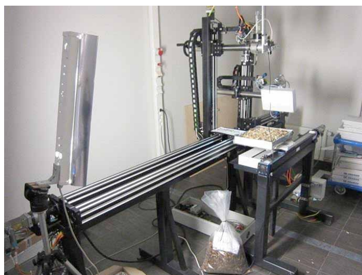
Figure 27. JAMK's machine vision test rig. Source: Juho Riekkinen.
