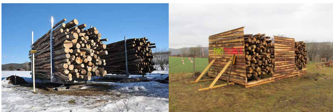
Figure 6. Austrian beech and oak stem wood drying trial 2013 (left) and beech stem wood drying trial 2014 (right) . Notice the wind wall in the picture on the right. Source: Gernot Erber.
