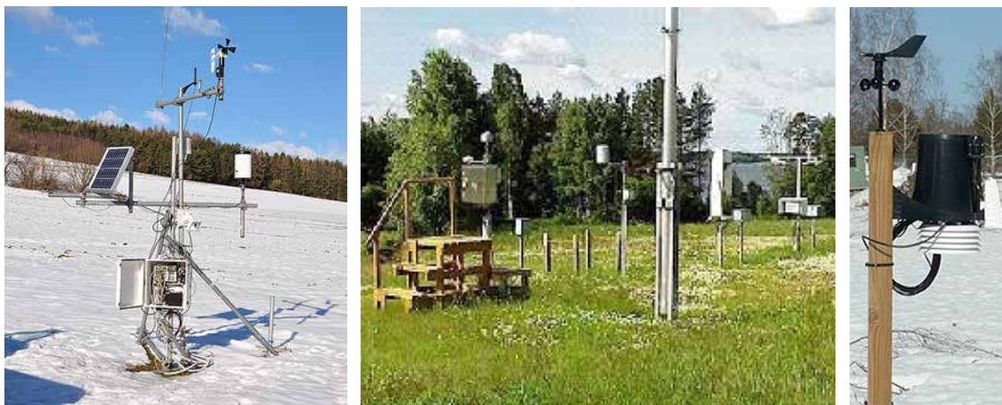
Figure 2: Meteorological station types used for the drying trials. Mobile, solar powered type at Austrian trial (left), stationary at the Finland A trial (middle), and a simple but functional “€ 1000 station” in Sweden (right). Source: Gernot Erber, UEF and Lars Wilhelmsson.
