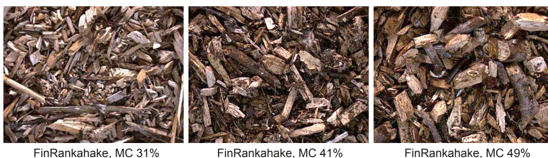
Figure 30. Finnish stem wood chips with differing moisture content.
