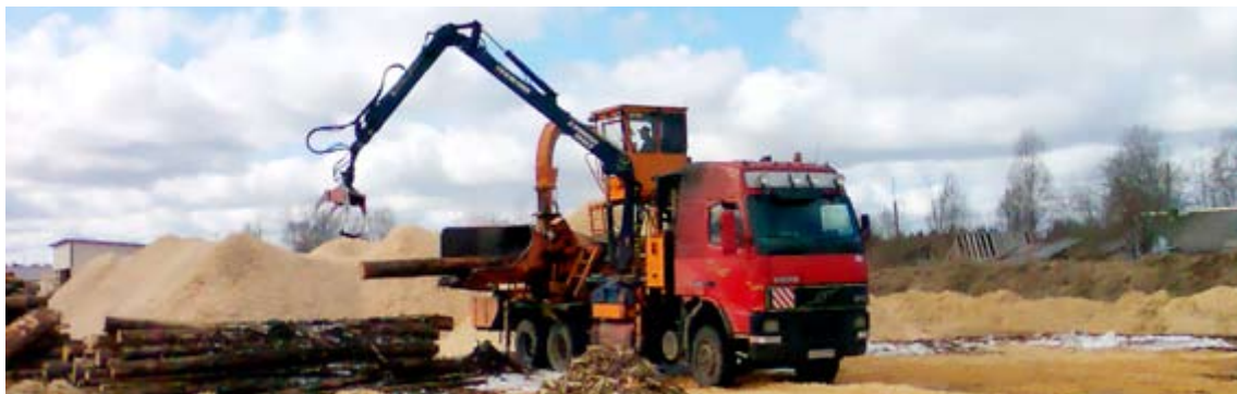
Figure 5. Mobile chipper Heinola 1310RML working on a terminal in the Republic of Karelia, Russia (photo: Y. Suhanov).
