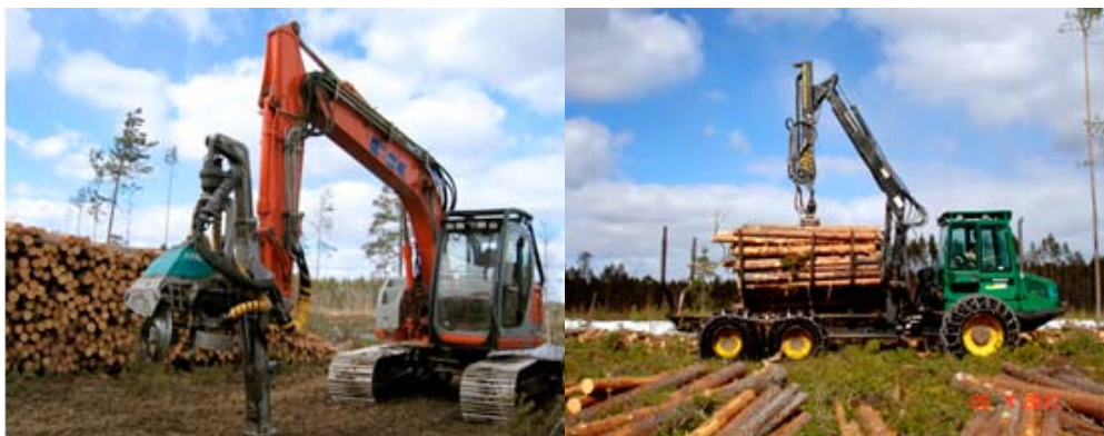
Figure 4. Excavator-based harvester Fiat-Kobelco E135SR (left side, photo: A. Seliverstrov) and forwarder Timberjack 1010D (right side, photo: V. Katarov).
