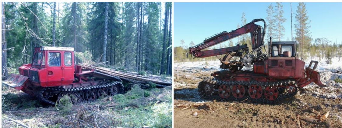
Fig. 3.34 Cable model of caterpillar skidder TLT-100A (left) and crane model of caterpillar skidder TB-1MA-15 (right).
