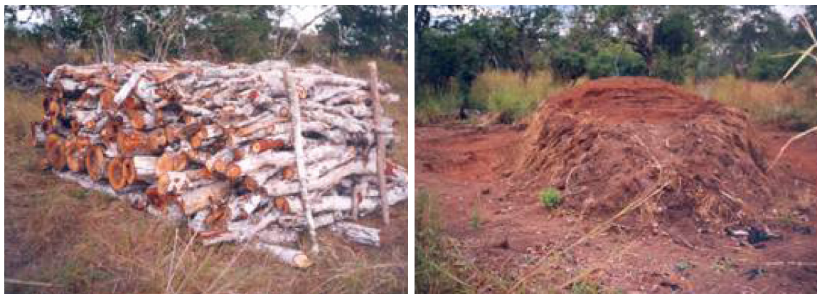
Figure 2. Typical earth mound charcoal kiln under preparation at Gwata area, in Morogoro.
