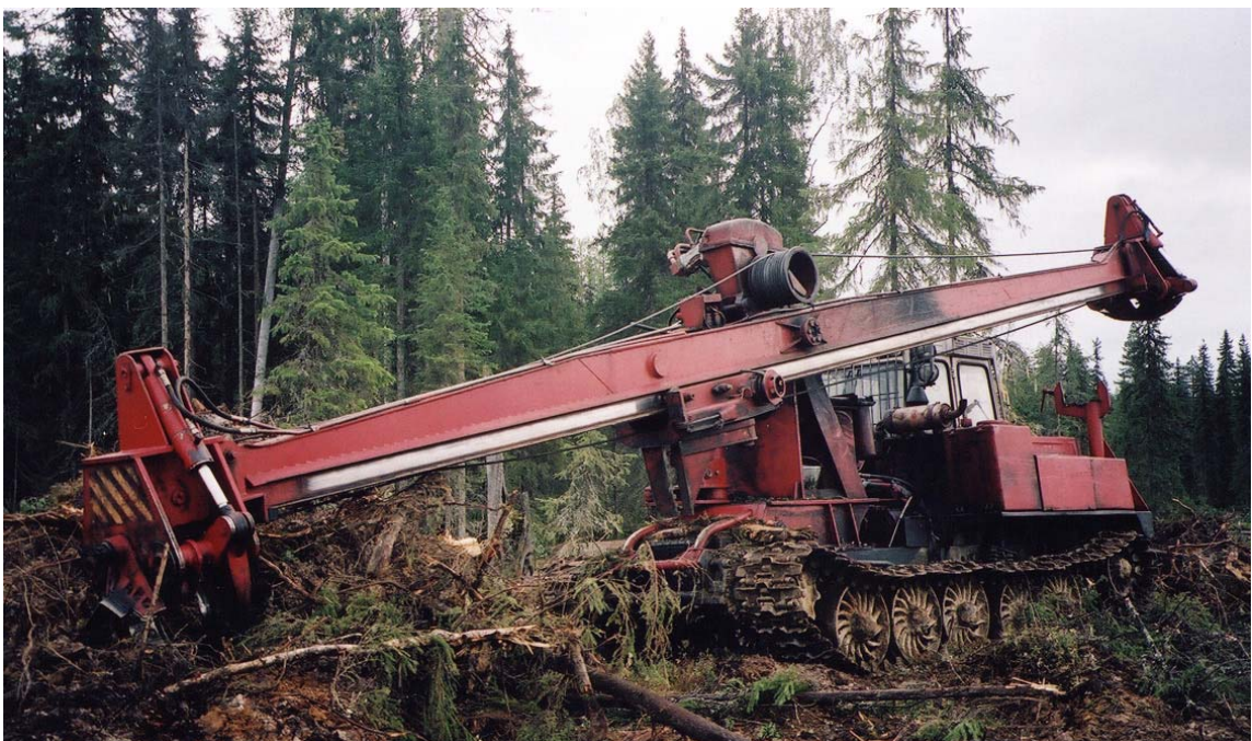
Figure 24. Delimiting machine LP-30. (Pavel Chikulaev)
