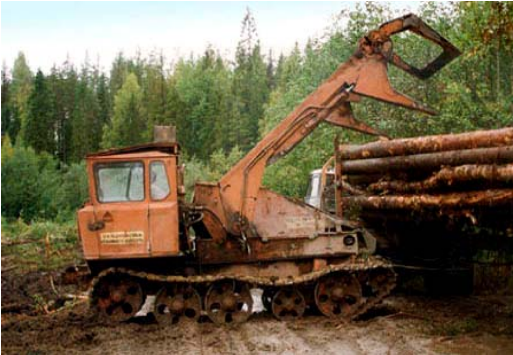
Figure 25. Loader PL-1V at the upper landing. (Lauri Sikanen)
