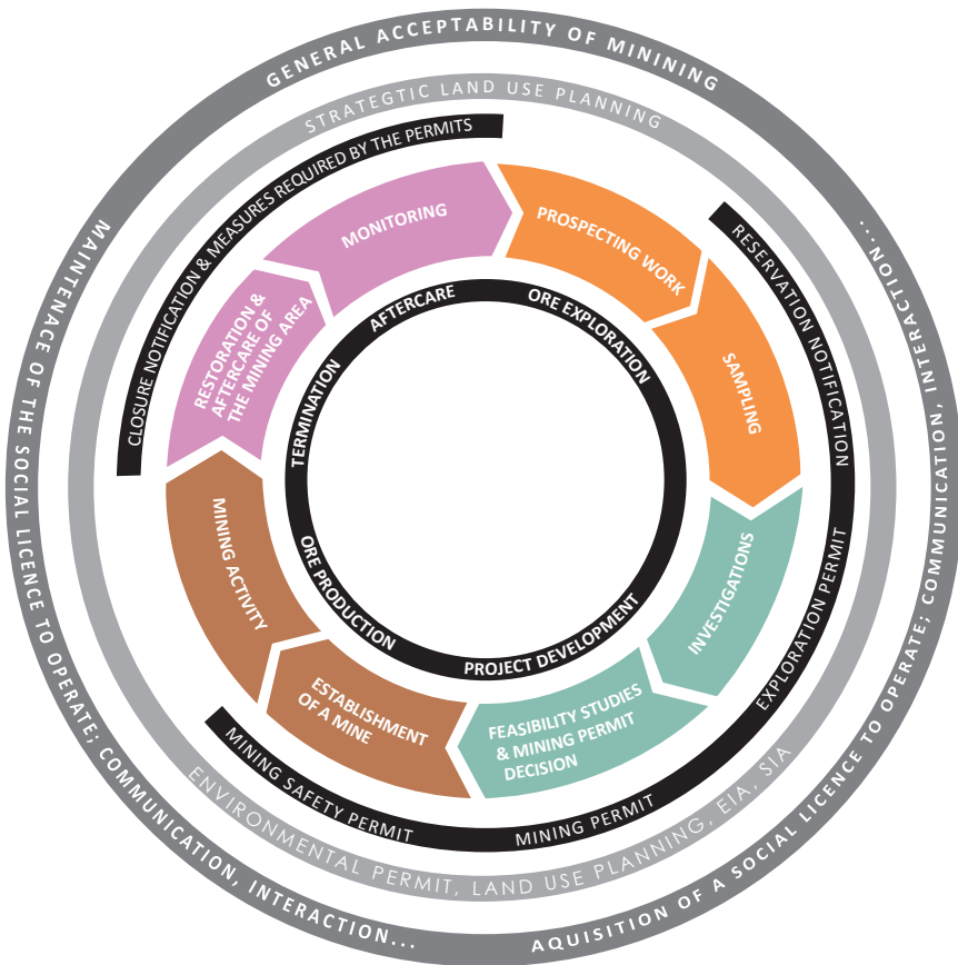
Chart 8. Environmental regulation and practices supporting the social sustainability of mining. Chart: Leena Soudunsaari, Helka-Liisa Hentilä, and Anniina Valjus.
