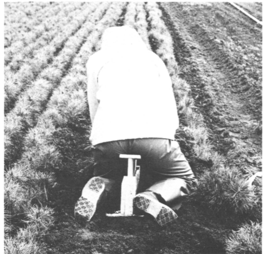
Fig. 24. Footstool that reduced the strain on the legs in the kneeling position
