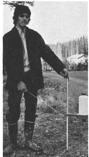
Fig. 5. The herbicide-granule spreader constructed by PENTTI NISULA. The container is placed above the young tree with the aid of an aluminium stick. When the string is pulled, the rotating mouthpiece under the container throws a fixed portion of herbicide grains around the tree. The height of the spreader can be adjusted by moving it along the stick. Photo P. NISULA.
