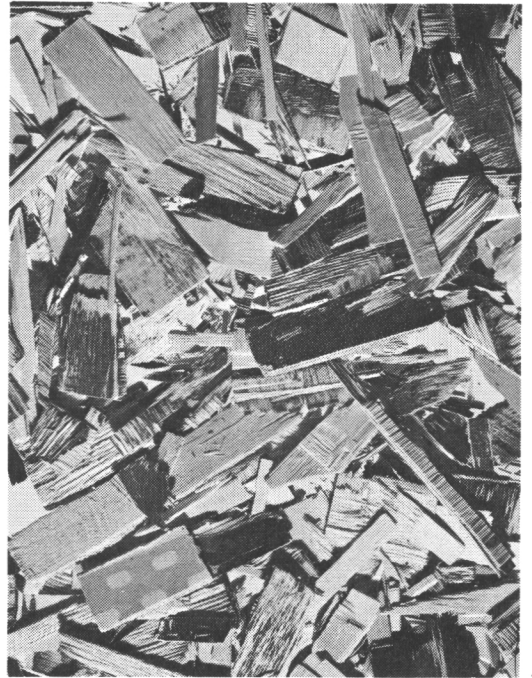
Fig. 1. Chips prepared from various kinds of plywood plant waste.
