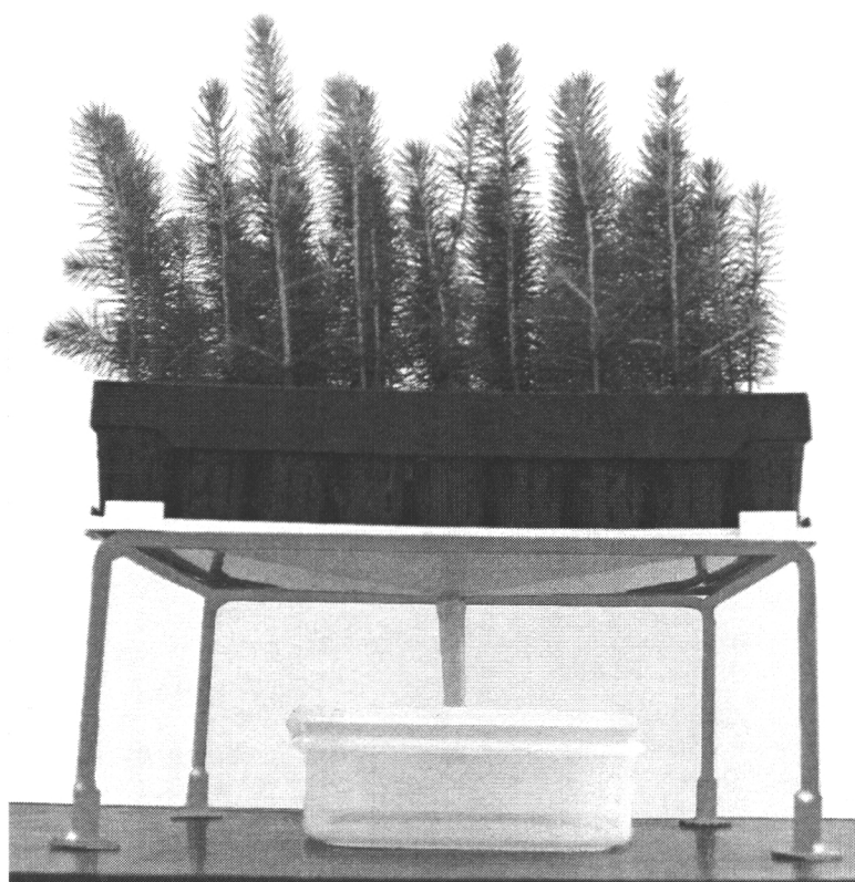
Figure 3. Leachate collector with plate and vessel. One-year-old Norway spruce seedlings in Plantek 81F container tray (photographed by Pekka Voipio).
