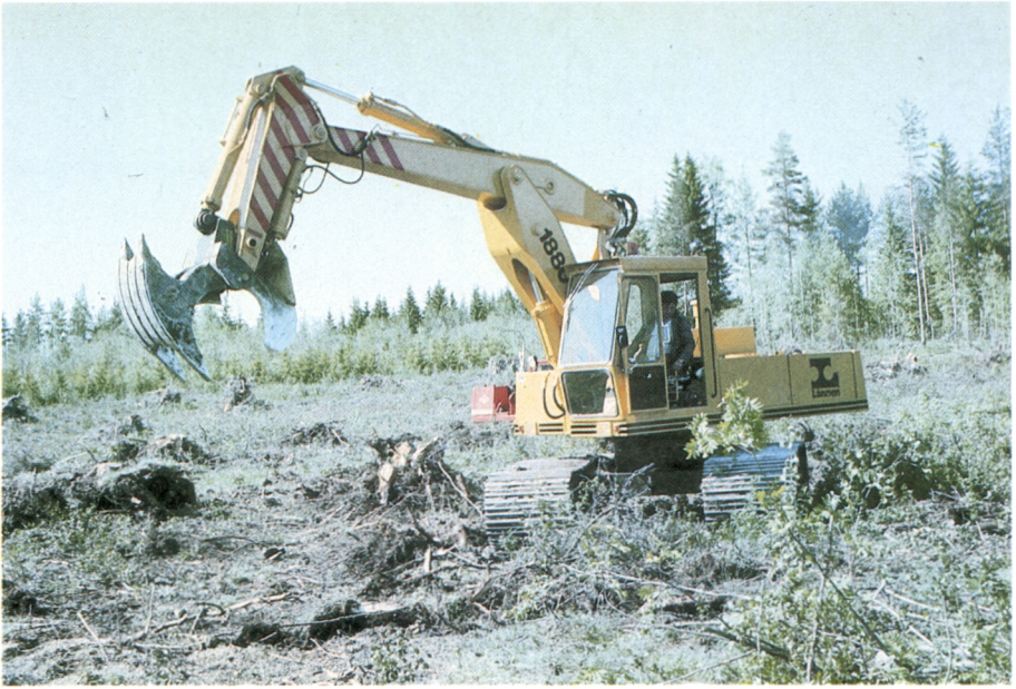
Figure 7. Harvesting of stump and root wood is being developed to get additional fiber material for the sulphate pulp industries.
