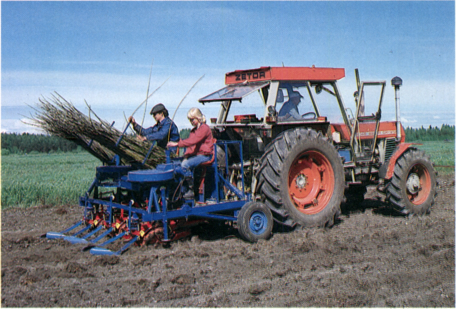
Figure 17. Developing planting techniques for willow cuttings for the establishment of short-rotation energy plantations.
