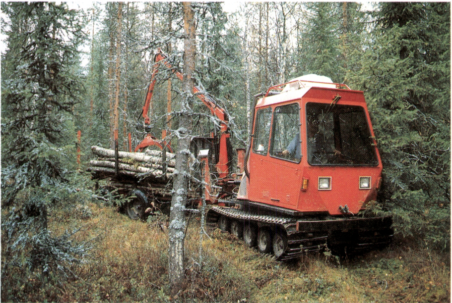
Figure 12. A research project on peatland logging gives special attention to development of machines with a very low ground pressure.
