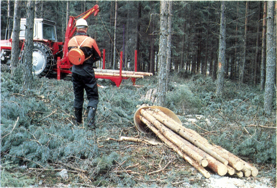
Figure 9. About 25 % of timber is sold delivered to the road side by the forest owner himself using farm tractor-based equipment.
