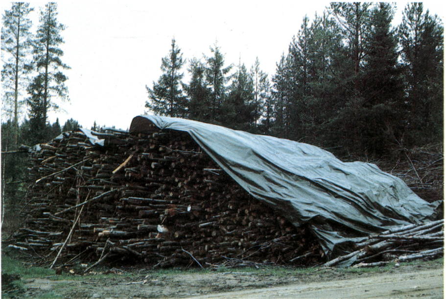
Figure 26. Different kinds of coverings are studied to decrease the moisture content of whole trees in winter.
