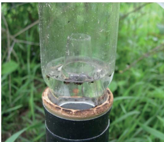
Fig. 13 and 14. Glass head box of the ground photo-elector in profile and top view with caught sea buckthorn fruit flies (Photos Höhne)
